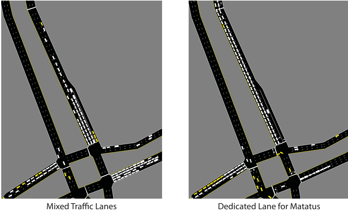
Figure 19. Queues on Uhuru Highway approaching University Way grow longer if a lane is dedicated to matatus, because less space is available on the street for the same number of private vehicles.
