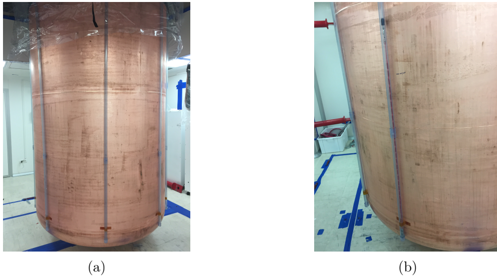
Figure 8.3: (a) View of the OVC with PVC pipes installed. The curving path can be seen at the top. (b) Close up of one source string deployed in the “calibration” position in its pipe.
