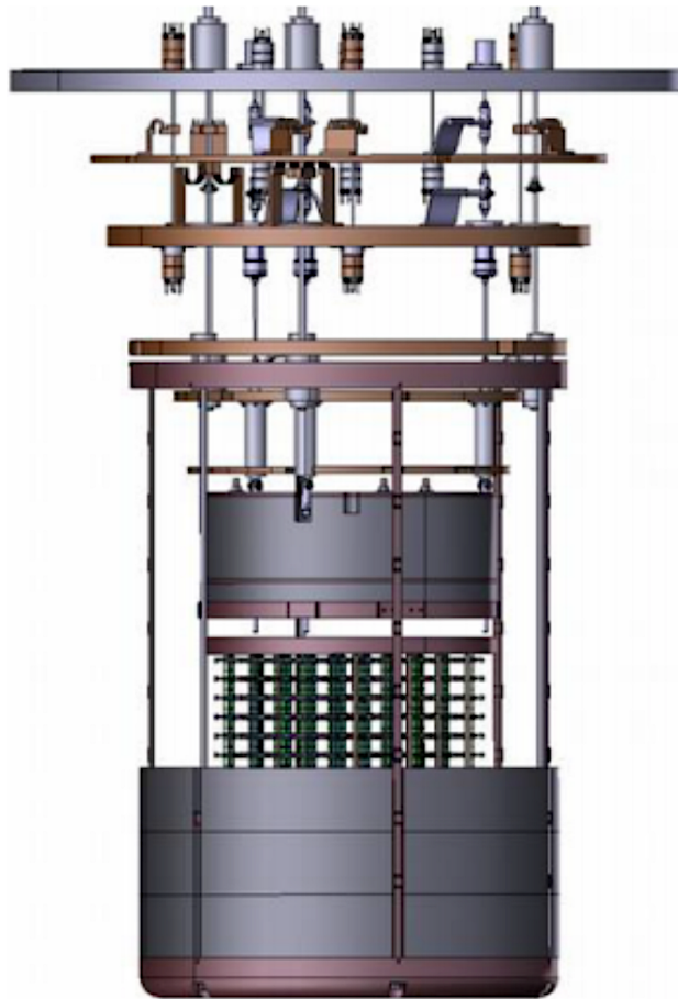
Figure 5.12: Side-view cutaway rendering showing the CUORE cryostat’s plate suspension and cold lead shields. Only the bottom third of the Roman lead side shield (4 K) is shown so that the detector, TSP, top lead shield (50 mK), Mixing Chamber plate (10 mK), and cold plate (100 mK) can be seen. Image credit CUORE Collaboration.
