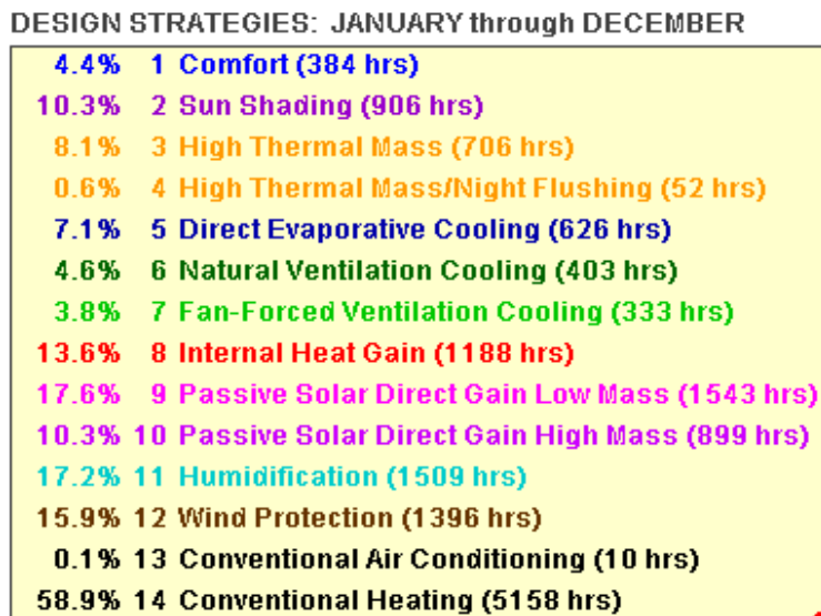
Fig.8: Design Strategies: The percentage of hours that fall into each of the 14 Design Strategy zones on the Psychrometric Chart shows which will be most effective. Here in Climate Zone 16, the High Sierras, the best cooling strategy is 3. High Thermal Mass, and the best passive heating strategy is 9. Passive Solar Direct Gain in a Low Mass Building. In this case the conflict can be removed by clicking on one of these Design Strategies to remove it, which will recalculate the percentages of all the others. Sun Shading, Internal Gains, Wind Protection, and Conventional Heating will not conflict with each other so should remain.
