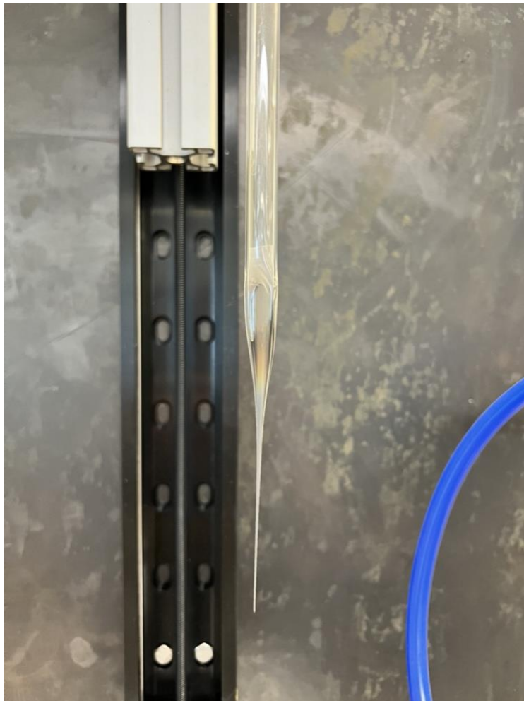
Figure 3.7- Initial Preform with 15mm SAM 2x5 Powder
