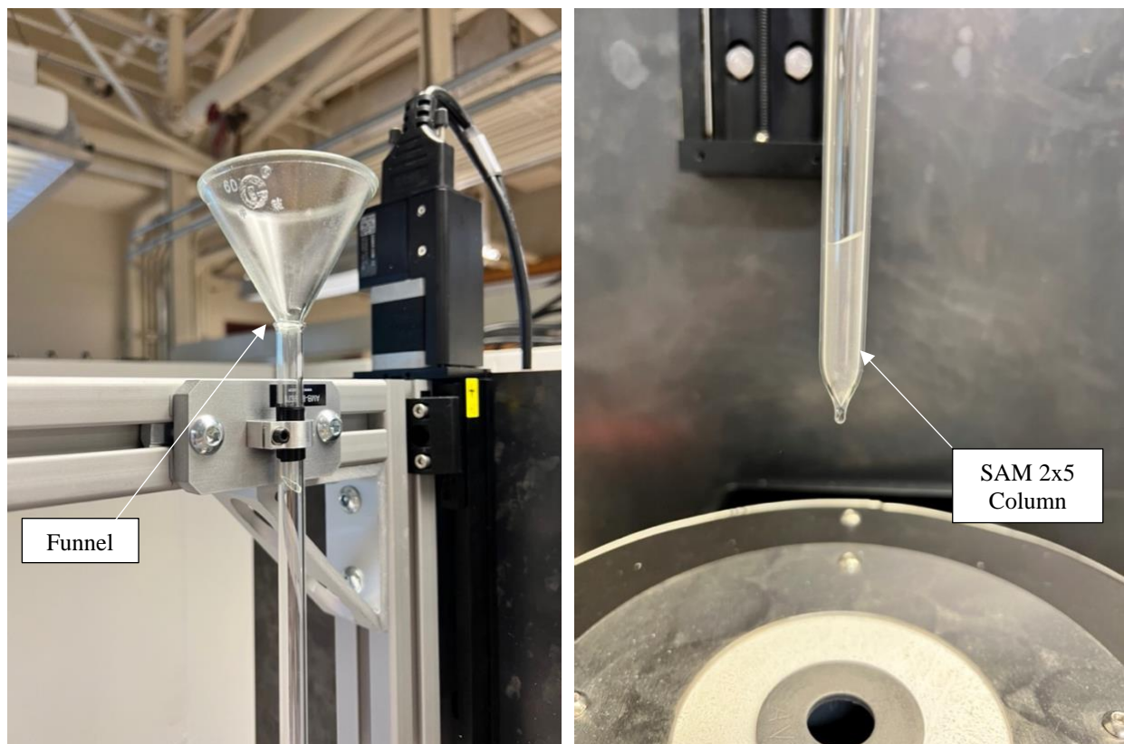
Figure 2.8- Addition of SAM 2x5 Powder to Preform
