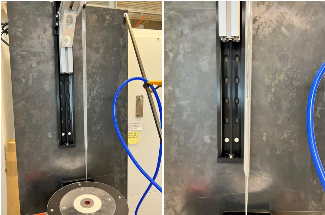
Figure 3.3- Initial Preform with 130 mm SAM 2x5 Powder
