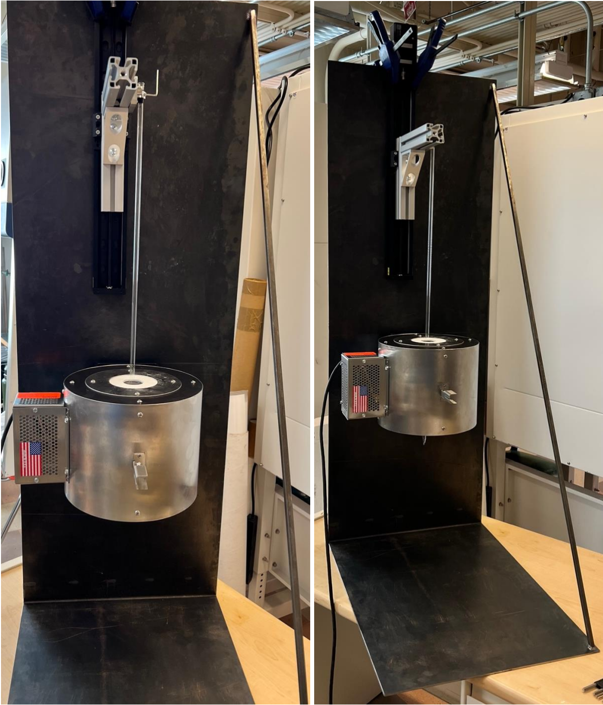
Figure 2.4- Centerline Test of Linear Slide Prior to Mounting
