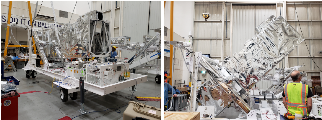
Figure 1.20 The PICTURE-C gondola being tested at CSBF in Fort Sumner, NM prior to its first flight in September 2019. The gondola is the large white structure holding the telescope that is covered by Mylar to reflect stray light at night and solar radiation during the day. (Left) A lift test being performed, hoisting the gondola up with the balloon mounting harness beneath an overhead crane. (Right) A pointing test with the PICTURE-C gondola where the telescope travels through its full range of motion.
