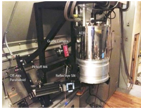
Figure 1.14 The ARCONS cryostat mounted at the Palomar 200" telescope Coudé focus. Also shown are several of the foreoptics (Pickoff M4, Off Axis Paraboloid, Reflective Slit) that enable the light to be directed into the instrument. Accessed via http://web.physics.ucsb.edu/~bmazin/projects/arcons.html .
