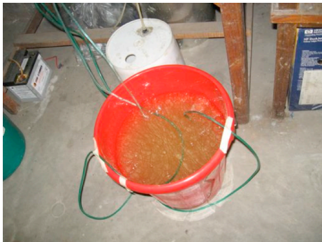
Photograph 3. ARUBA particle suspension through aeration.
