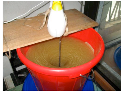
Photograph 4. ARUBA particle suspension with a mechanical mixer.
