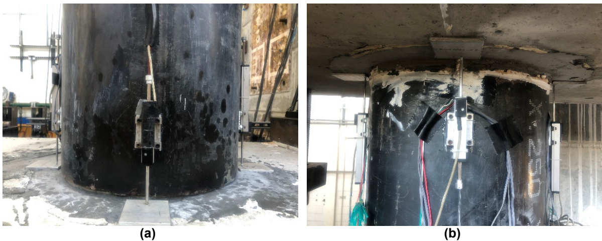
Figure 6.35 (a) LVDTs installed at the bottom interface; and (b) those at the top interface.
