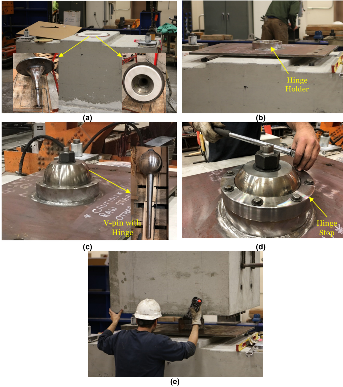
Figure 3.15 V-connector assembly sequence: (a) place the Teflon washer; (b) put on the top steel pad; (c) insert the V-pin; (d) attach the hinge stop; (e) set up the top block.
