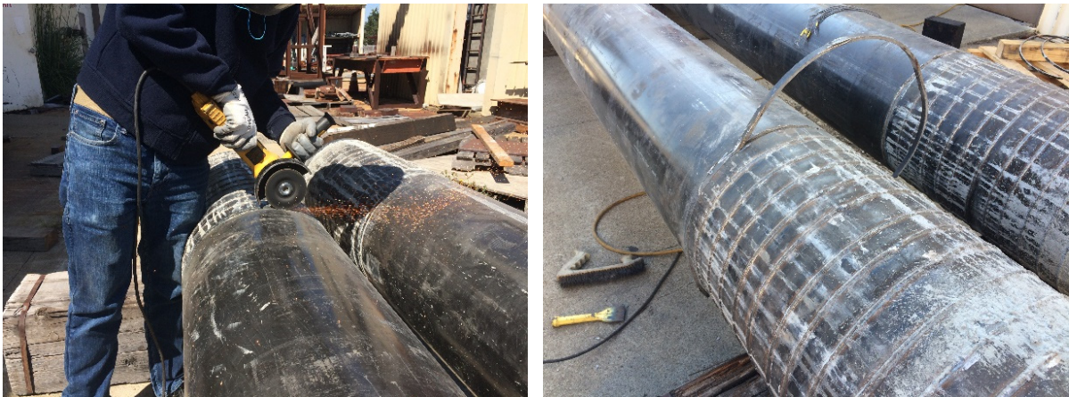
Figure C.3 Remove the 0.25 in. steel strips at the column rocking interfaces.
