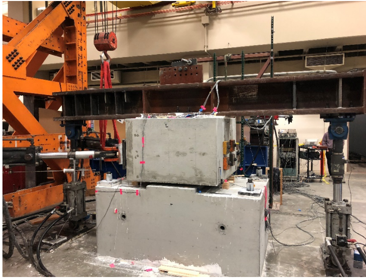
Figure 3.8 Test setup for the V-connector experiments.
