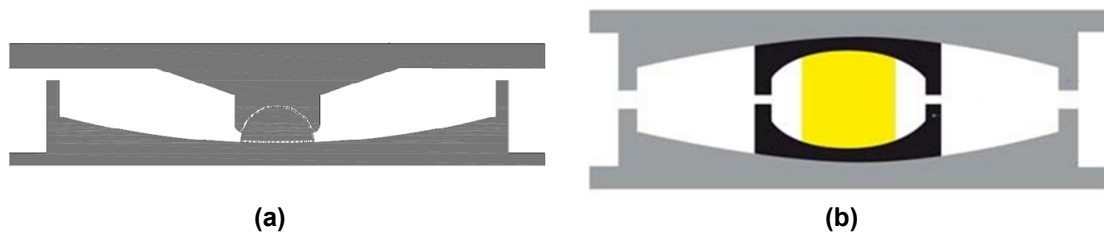
Figure 2.3 (a) Single friction pendulum bearing; and (b) triple friction pendulum bearing (source: Google Images).
