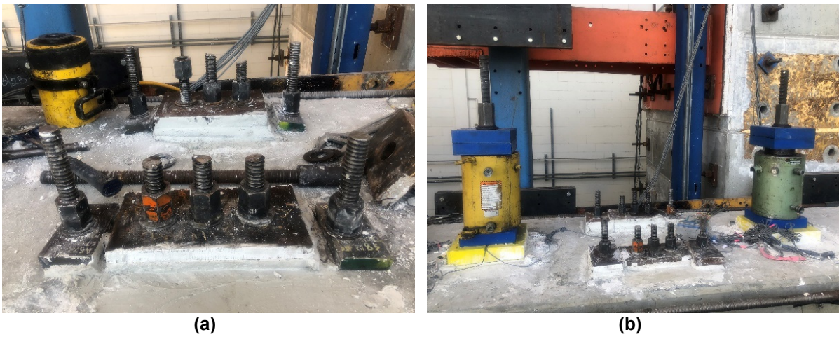
Figure C.13 (a) Top view of the vertical actuator connection rods; (b) set up the prestressing jacks and prestress the PT bars to 40% GUTS.
