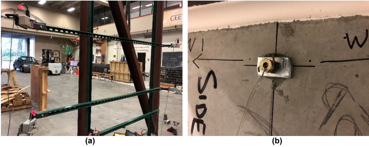
Figure 3.18 (a) WPs on the east-side instrumentation frame; (b) target point attached to the reinforced concrete block surface.
