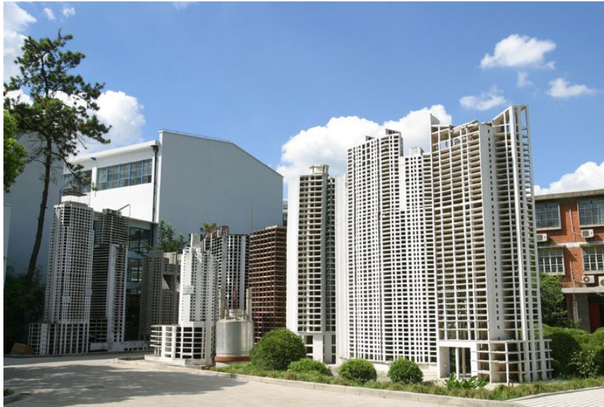
Figure 2.10 Reduced-scale buildings for shaking table tests in Tongji University, China (source: Google Images).
