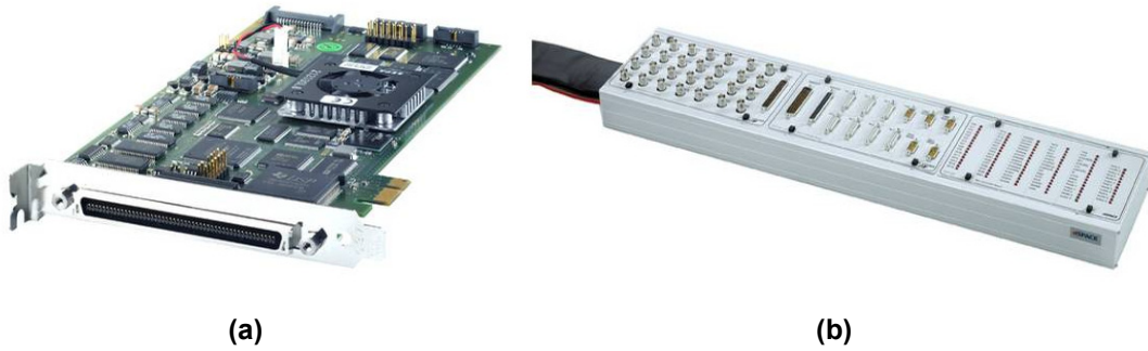
Figure 7.14 (a) DS1104 R&D Controller Board; (b) CP1104 connector panel with ADC and DAC channels (source: Internet).
