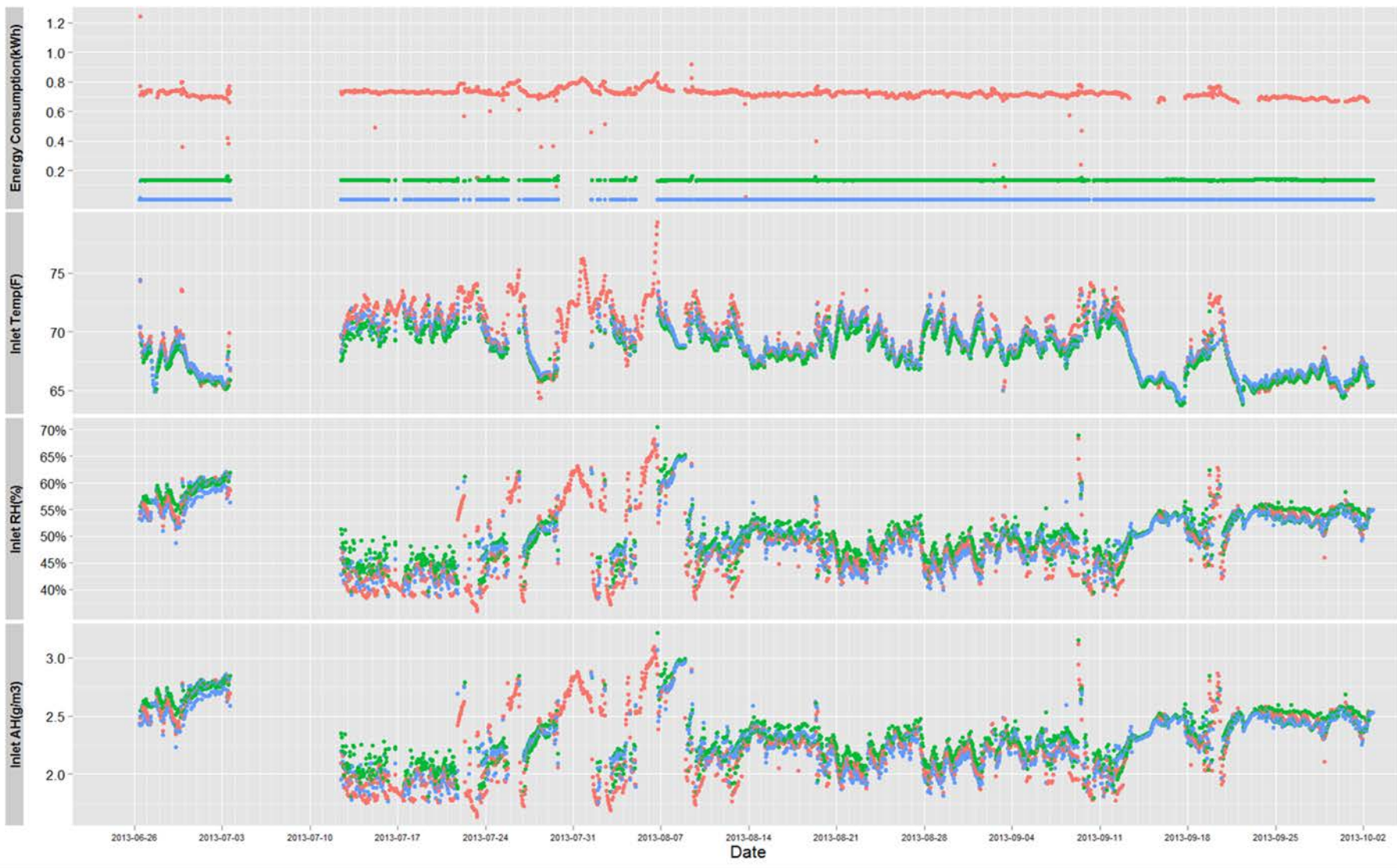
Figure 4-15 Hourly Profiles of Energy Use, Temperature, RH, and Absolute Humidity at the Air Inlet for WHD-Site03
