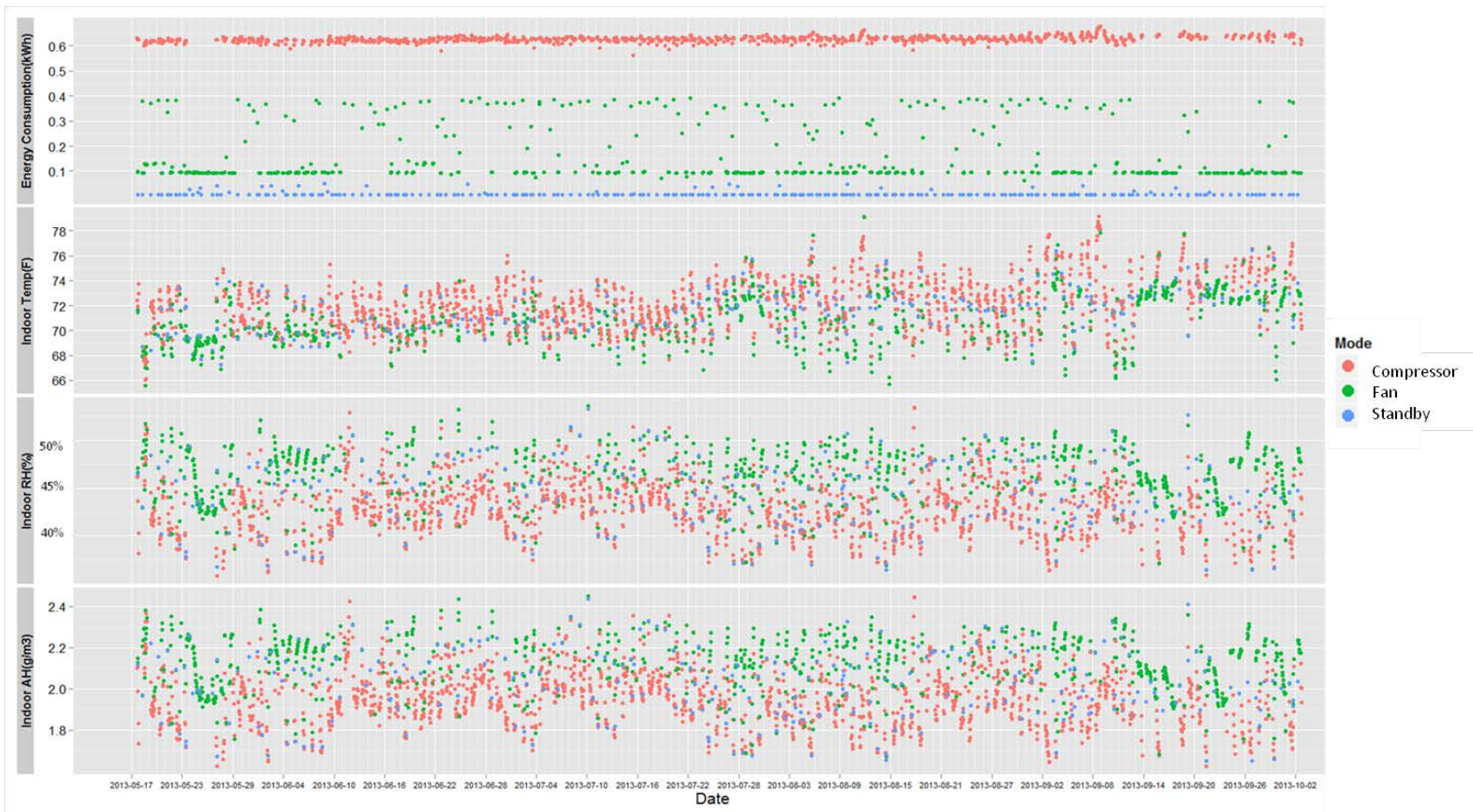
Figure 4-1 Hourly Profiles of Energy Use, Temperature, RH, and Absolute Humidity at the Air Inlet of WHD-Site01
