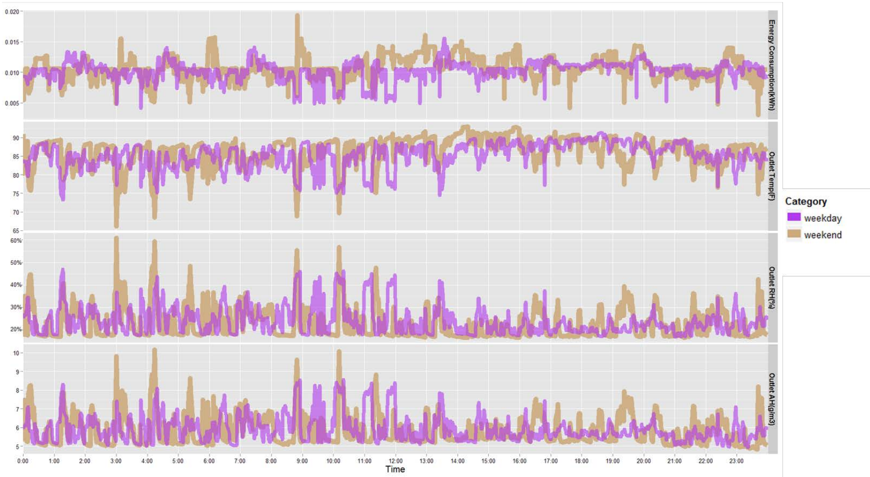
Figure 4-11 Average 24-Hour Profiles for Energy Use and Outlet Temperature, RH, and Absolute Humidity During Weekdays and Weekends for WHD-Site02
