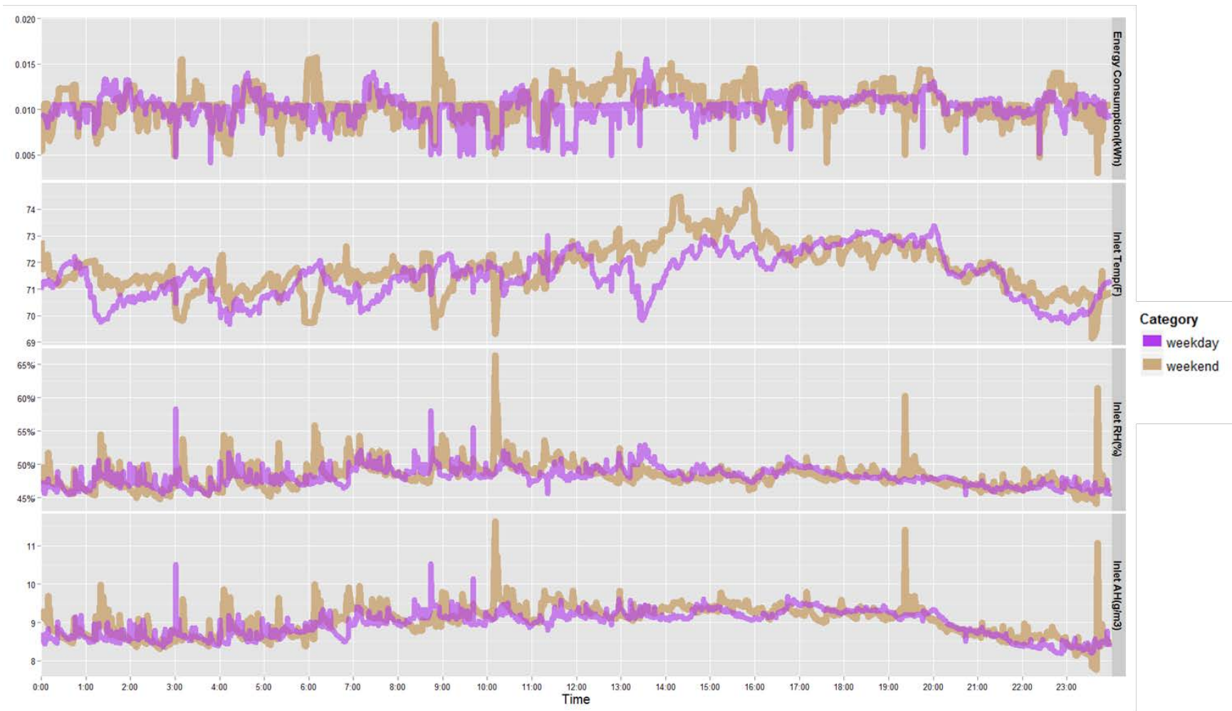
Figure 4-10 Average 24-Hour Profiles for Energy Use and Inlet Temperature, RH, and Absolute Humidity During Weekdays and Weekends for WHD-Site02
