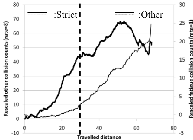
Figure 9. Oblique Cumulative Collision Counts Based on the Strict Definition
