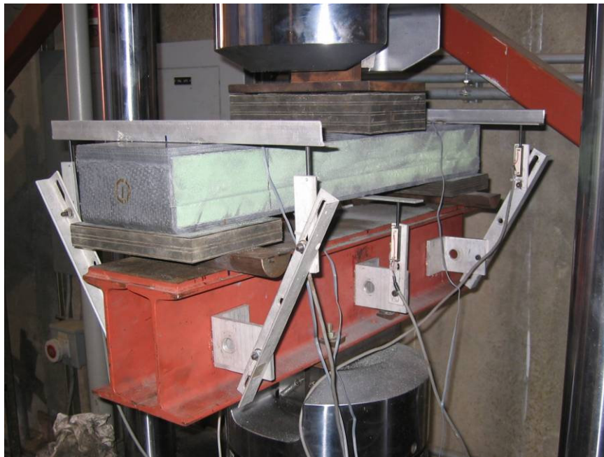
Figure 9-3 Photograph of the three-point bending test.
