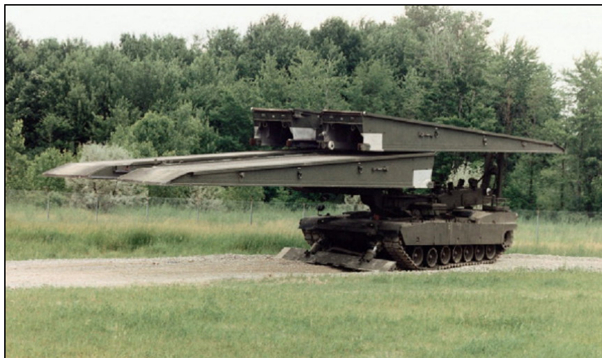
Figure 8-3 Photograph of the Wolverine Heavy Assault Bridge being launched.
