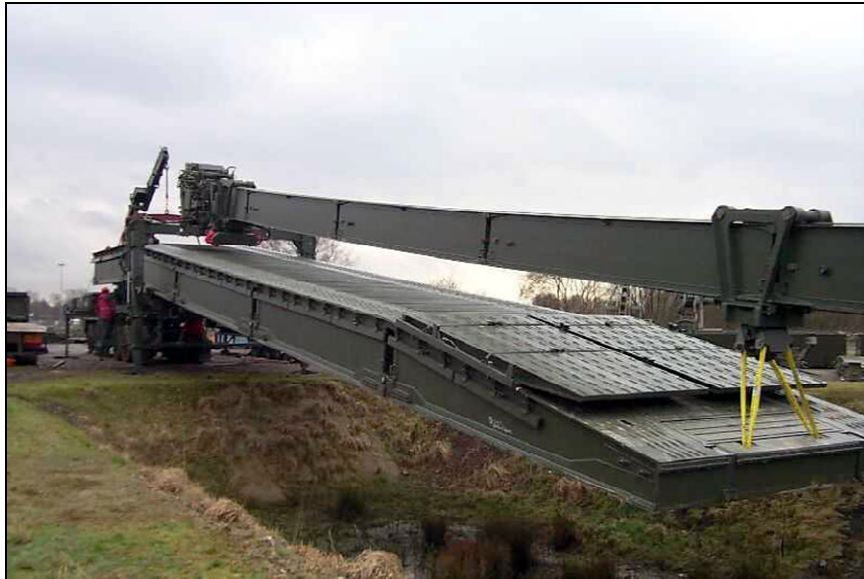
Figure 8-10 Photograph showing the DSB being launched across a gap.
