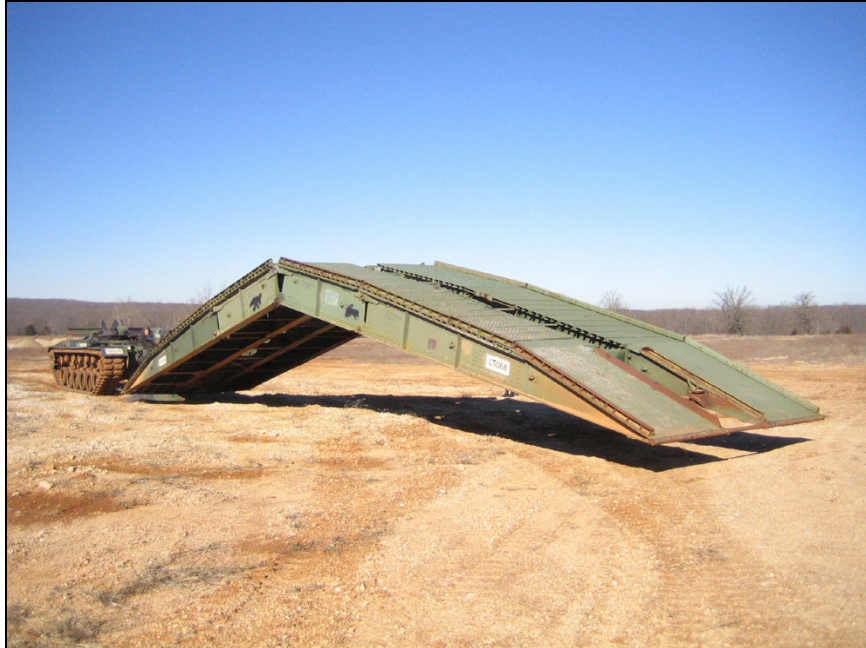
Figure 8-2 Photograph of AVLB being launched.
