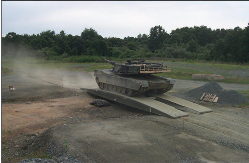
Figure 8-15 Photograph of an M1 Abrams tank crossing the Compos Army Bridge (CAB).
