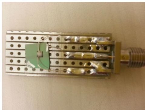
Figure 21 - Image of a Nickel on PZT sample inside of handmade packaging. Packaging is attached to a standard mini-SMA connector to allow for easy AC or DC biasing/measurement. The connector is attached to a proto-board and connector wires are soldered to the proto-board. To insure good connection between the package and substrate a standard ohmmeter is used to check continuity.
