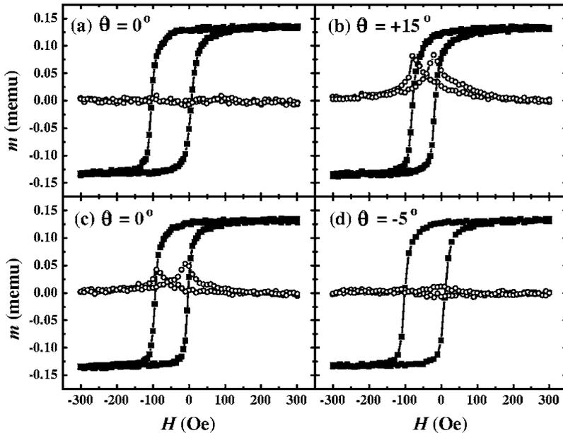
FIG. 1. Longitudinal loops (filled squares) and transverse loops (open circles) for FeMn (60 Å)/Co (100 Å) when the applied field is along  $\theta=(a) 0^\circ$ , (b)  $15^\circ$ , (c)  $0^\circ$  again, and (d)  $-5^\circ$ . The exchange field direction has rotated away from  $0^\circ$  after the field rotation.
