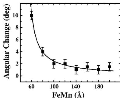
FIG. 3. FeMn film thickness dependence of the rotational hysteresis. The line is a fit to a modified inverse thickness dependence described in the text.
