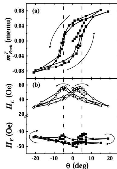
FIG. 2. Angular dependence of (a) the transverse peak height  $m_{\text{peak}}^T$  and (b) coercive and exchange fields for an FeMn (60 Å)/Co (100 Å) sample. The transverse peaks vanish at  $\theta=\pm 5^\circ$ , coinciding with the maximum coercivity in (b) and indicating a rotational hysteresis of  $10^\circ$  (dashed lines).
