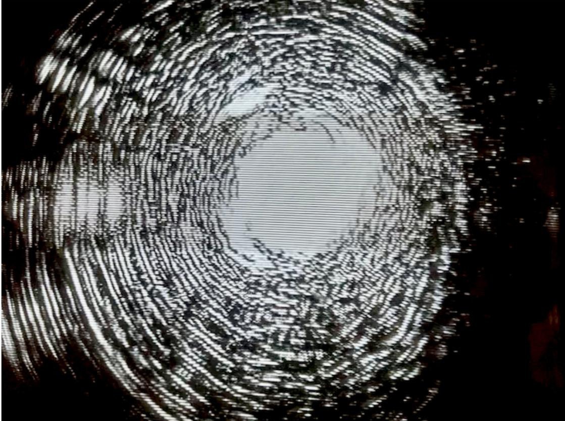
Figure 33: Screen capture from the video camera used on the output of the Fabry-Perot cavity while locking to the TEM<sub>00</sub> mode.
