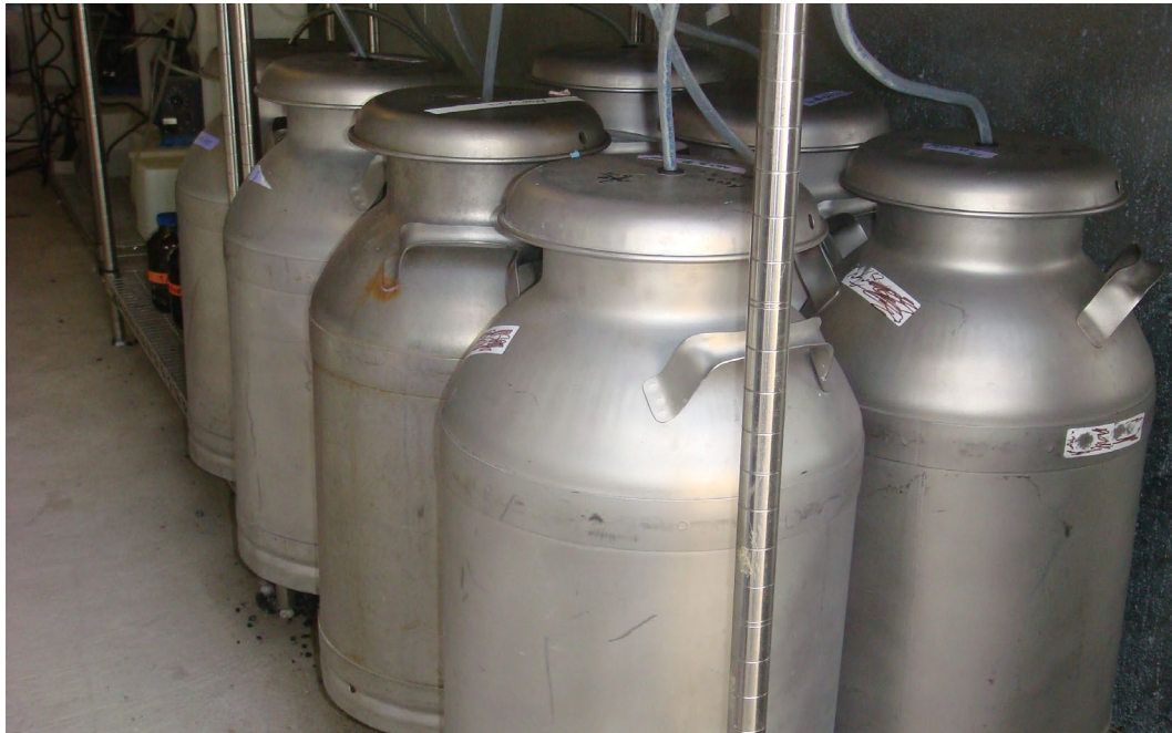
Figure 3-10 Photo view of the stainless steel composite water container
