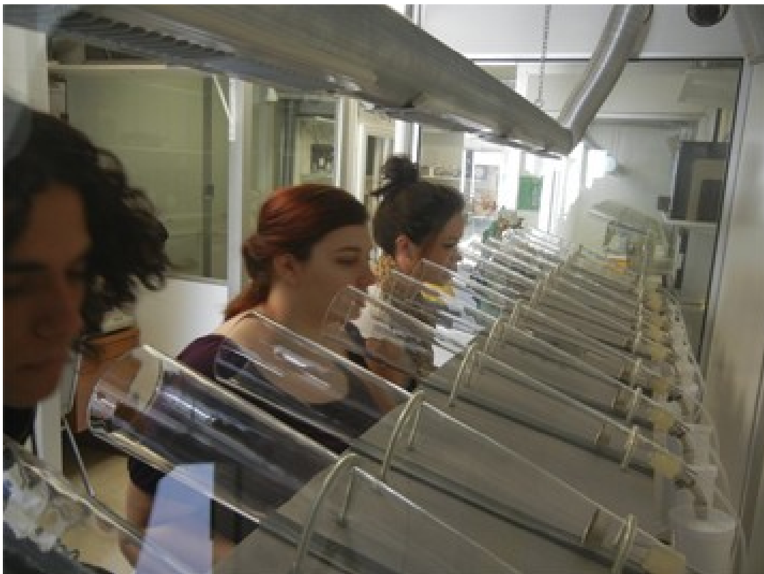
Figure 3. Subjects sniffing the cones of the VDD8 during test day. There is a computer controlled speaker system to control the timing.
