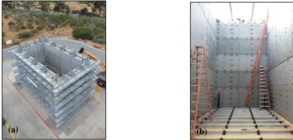
Figure 5. (a) General view of the NEES Large Soil Confinement Box and (b) inside view of the LSCB showing the fixed iron angles at the shake table platen.
