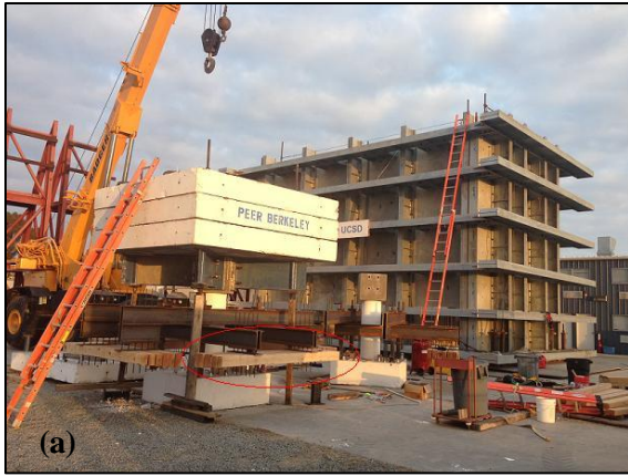
Figure 2. (a) Picture of the assembled aligned specimen and (b) reinforcing steel cage for the footing and the column.
