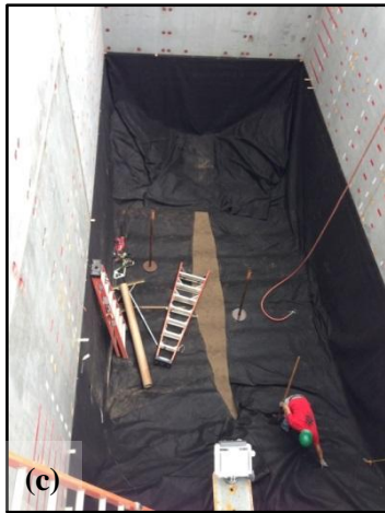
Figure 6. (a) Wetting and hand compaction the base soil into a curvy surface, (b) placing the geotextile at the sides of the box up to an elevation of 3.06 m, (c) general view of the installed geotextile and (d) general view of the lowered down liner system.
