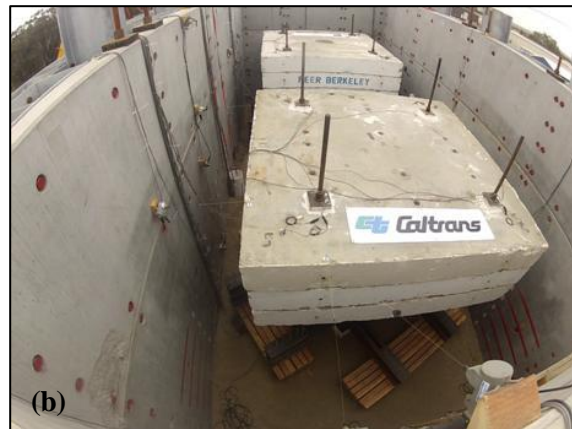
Figure 3. (a) Picture from inside the soil box after the placement of the specimens and (b) final configuration before test 1.
