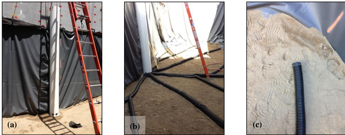
Figure 7. (a) Vertical PVC pipe used to insert and pump out water during saturation and desaturation process, (b) horizontal perforated pipes extending radially from the vertical pipe used to spread the water across the box plan view and bottom-up saturate the soil and (c) close picture of the perforated pipes.
