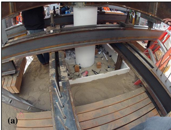
Figure 3. (a) Picture from inside the soil box after the placement of the specimens and (b) final configuration before test 1.
