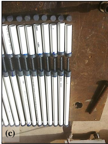
Figure 17. (a) Hex bushing attached at the bottom of outer PVC pipe with neoprene rubber wrapped around, (b) placed and secured against cage and formwork outer mechanisms for aligned footing before casting, (c) constructed internal mechanisms, (d) view of the installed gap-no gap instruments for aligned footing and (e) bottom view of skew footing while flying specimen in the box showing pattern and deflection of gap-no gap instruments.
