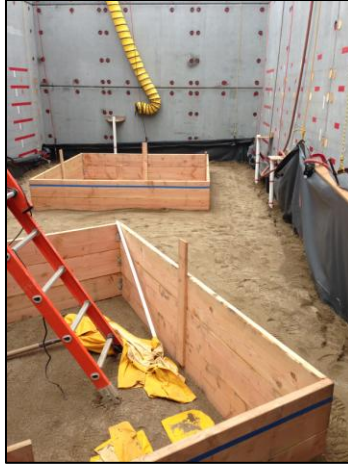
Figure 9. View of the temporary wooden frames used to allow placement and compaction of most of the soil above the foundation elevation prior to the placement of the specimens.
