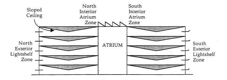
Figure 1: Cross section of five story building showing unique features, light shelves, sloped ceiling, and atrium.
