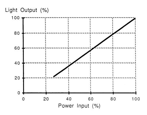
Figure 4: Plot of the relative change in input power for change in the light output.
