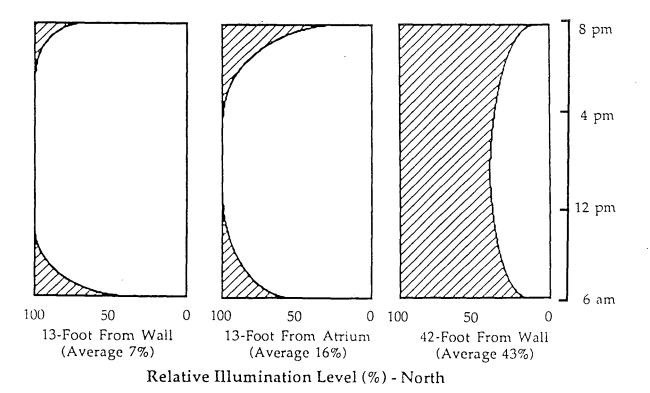
Figure 3: Daylight illumination levels during a working day in the north and South wings at three depths measured from the outer envelope or atrium.
