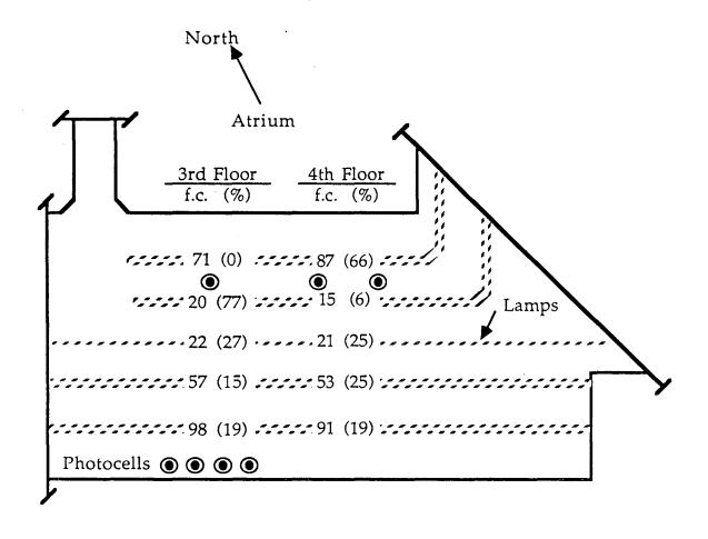
Figure 5: Relative decrease in the input power (parentheses) for rows of lamps and the measured daylight illumination levels on the south wing of the third and fourth floors.
