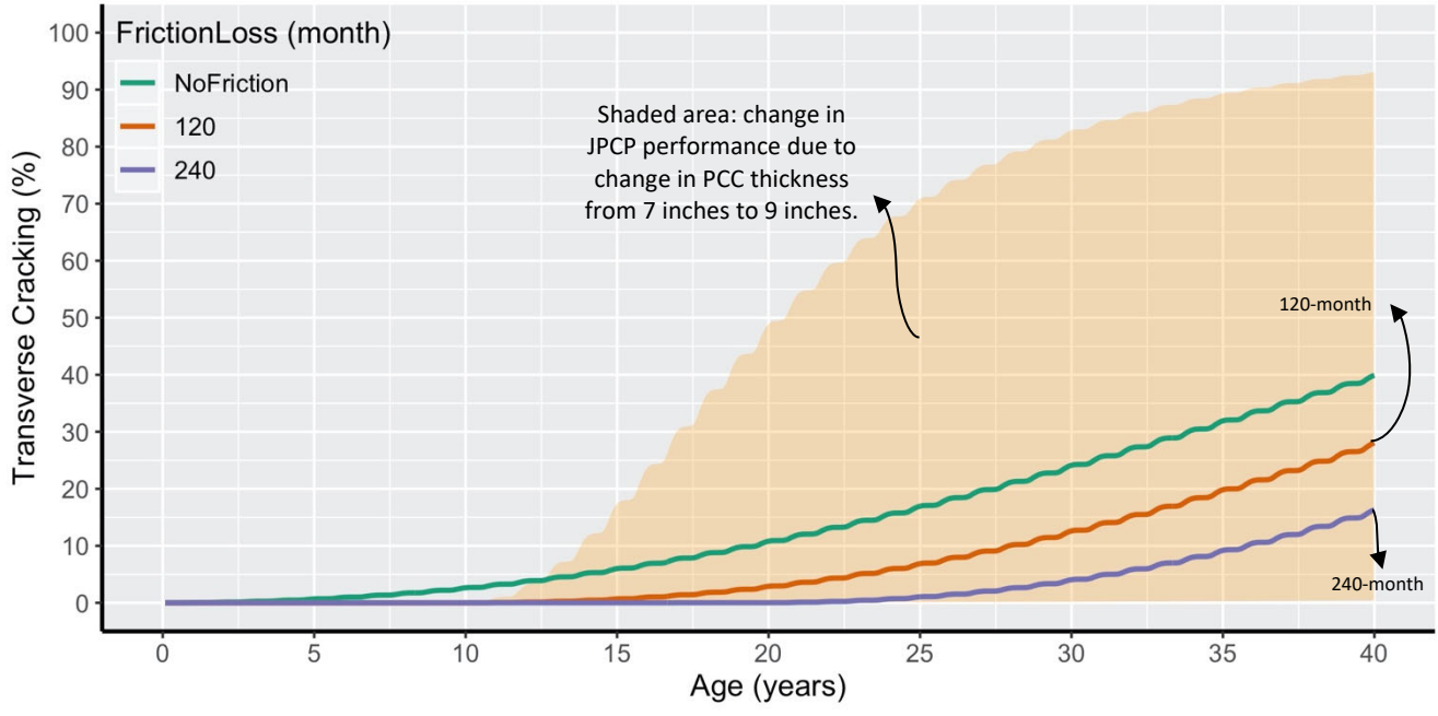
Figure 4.11: Effects of friction loss duration on transverse cracking with 50% reliability.
