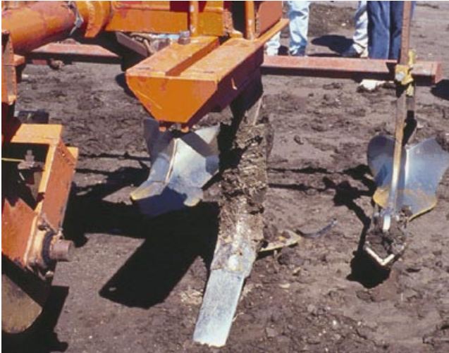
Figure 5. Minimum-tillage ripper for use in the Salinas Valley on permanent beds to break compacted layers to approximately 20 inches (50 cm) deep with angled, broad shanks and floating wings.
