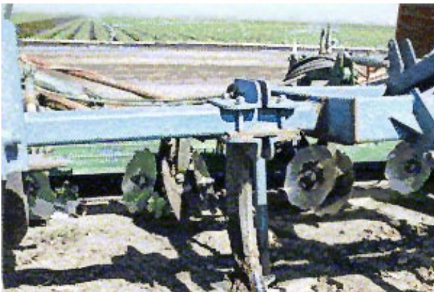
Figure 4. Minimum-tillage chisel for use in the Salinas Valley on permanent beds to simultaneously disk-hill the beds and chisel the furrows to approximately 20 inches (50 cm) deep with a narrow shank.
