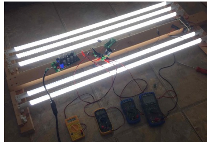
Zone Light, 380 V DC, 6% W saved
