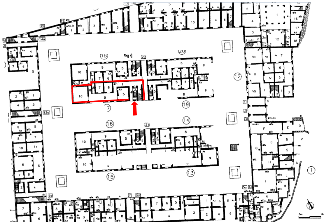
Figure 3.13. Plan of apartment complex in ancient Ostia, Italy. A single unit is outlined in red, with an arrow indicating the entryway for both groundfloor and upper stories: this floorplan repeats with minor variation for the other units, as well as those which would have stood above. Each unit is similar in plan to the example from figure 2.11. (Image based on Cervi 1998, figure 2.)
