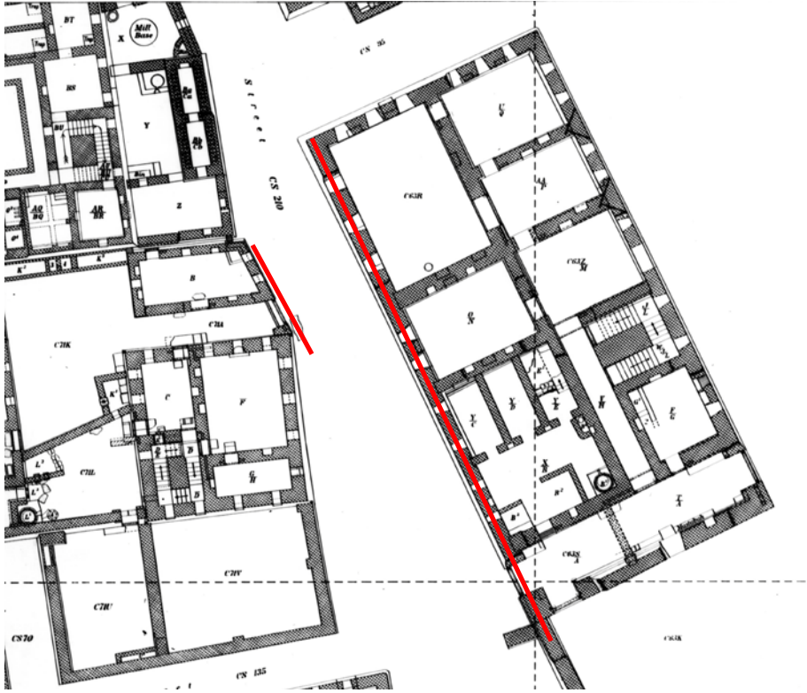
Figure 4.8. Structures to the east of CS210 follow the orientation of C63, which probably predates the structures to the west. Buildings of the west side follow the overall orientation of KAC, but here a few walls are angled (in red) so as not to narrow street access.
