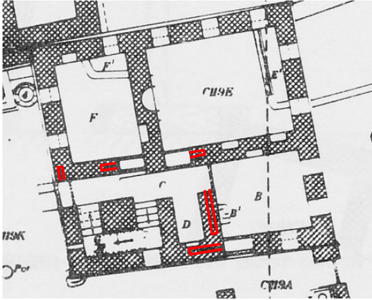
Figure 5.15. Above left, line drawing of the door bolt resting in its channel inside the house wall. Above right, decorative exterior case for the door bolt, here in the shape of a naos. Below: house C119, with door-bolt channels located in nearly every doorway, here outlined in red for clarity.
