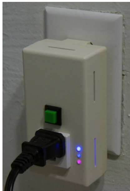
Figure 13: ACme outlet energy monitor and controller.
