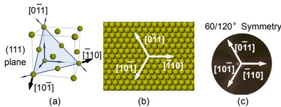
FIGURE 4. (a) (111) PLANE IN FCC CELL, (b) (111) PLANE, (c) SURFACE CHEMICALLY ETCHED (111) WORKPIECE.
