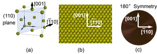
FIGURE 3. (a) (110) PLANE IN FCC CELL, (b) (110) PLANE, (c) SURFACE CHEMICALLY ETCHED (110) WORKPIECE.
