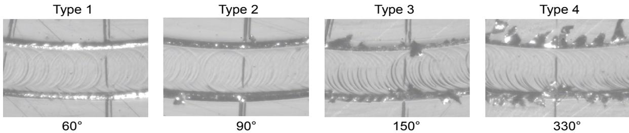
FIGURE 7. SINGLE CRYSTAL BURR CLASSIFICATIONS IN SLOT MICROMACHINING (110 WORKPIECE,  $f_t = 1 \mu\text{m}$ ,  $v_c = 12.75 \text{ m/min}$ ).
