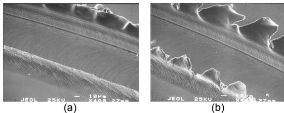
FIGURE 8. SEM IMAGES OF BURR SHAPES VARIATION ON (100) PLANE AT (a)  $135^\circ$  AND (b)  $180^\circ$  ( $f_t = 1 \mu\text{m}$ ,  $v_c = 17 \text{ m/min}$ ).
