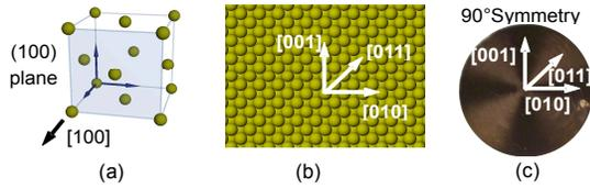
FIGURE 2. (a) (100) PLANE IN FCC CELL, (b) (100) PLANE, (c) SURFACE CHEMICALLY ETCHED (100) WORKPIECE.
