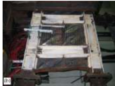
(b) Specimen no. 5 with stiffened infill plate and simple beam-to-column connections
