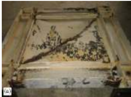
(a) Specimen no. 1 with unstiffened infill plate
