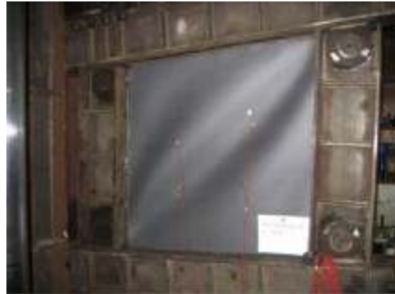
(b) Buckling of unstiffened specimen
