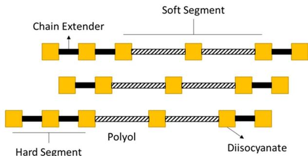
Fig. 1 Chemical structure of thermoplastic polyether polyurethane. The molecular structure of TPU comprises of three main segments: (1) isocyanate, (2) polyol, which may be polyester, polyether, or polycarbonate, and (3) a chain extender. The reaction of these components forms a morphology known as a segmented structure, including alternating soft and hard segments. The combination of the chain extender and diisocyanate forms the hard segments, while the polyol component forms the soft segments.
