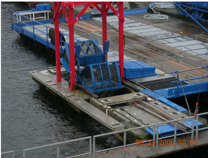
Figure 1: A version of Ito's fish wheel remains in use today near Chitose, Hokkaido. (Photo by author)
