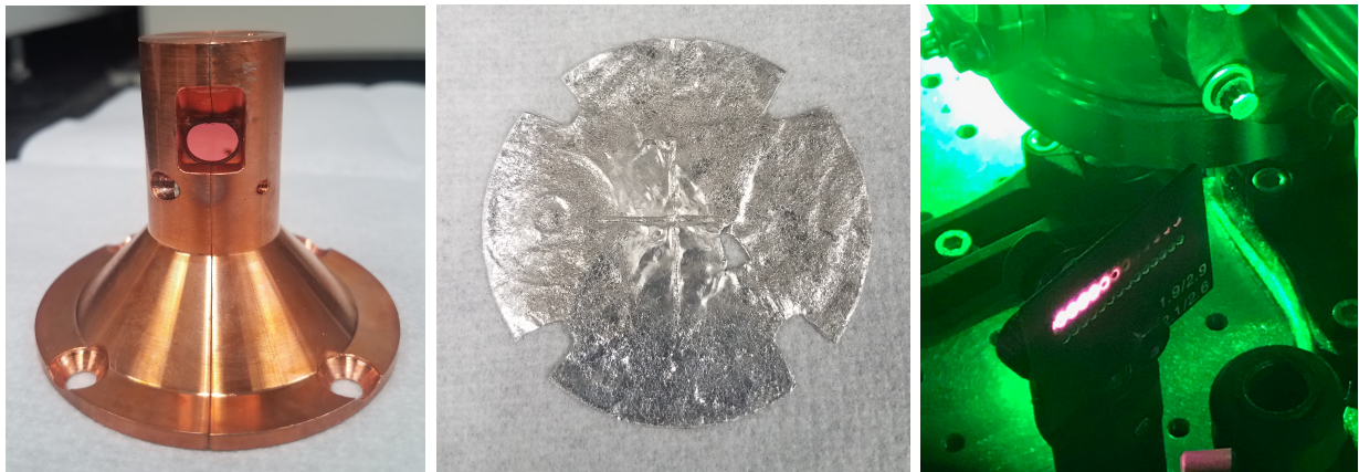
Figure 2.4: Left: Mounted amplifier crystal. A small burn can be seen on the bottom right corner of the crystal. Center: Indium foil cut to fit the amplifier crystal mount. Right: Aperture mask with fully amplified beam. Increasing beam divergence can be seen with successive passes (right to left).
