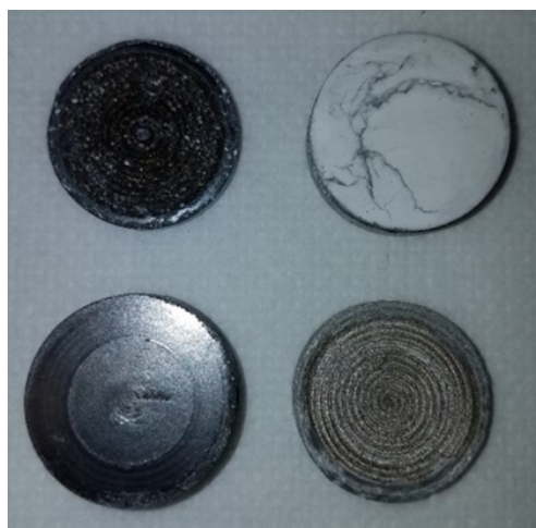
Figure 9.4: Homemade pressed uridine targets after irradiation. Clockwise from top right: neat uridine pressed by 20 T, 1:1 by volume indium:uridine pressed by 12 T, 1:1 by volume carbon:uridine pressed by 20 T, 2:3 by volume carbon:uridine pressed by 12 T.
