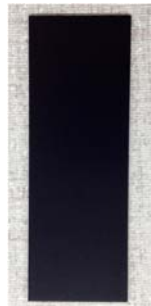
Figure 1: The MWNT-based film was sprayed onto a 75×25 mm 2 glass microscope slide before conducting water treatment.
