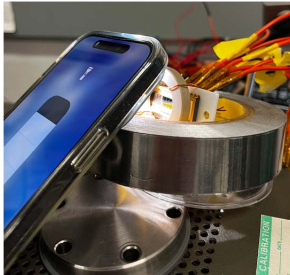
Figure 28: The polychromatic light testing setup, using different light intensities from a phone flashlight.
