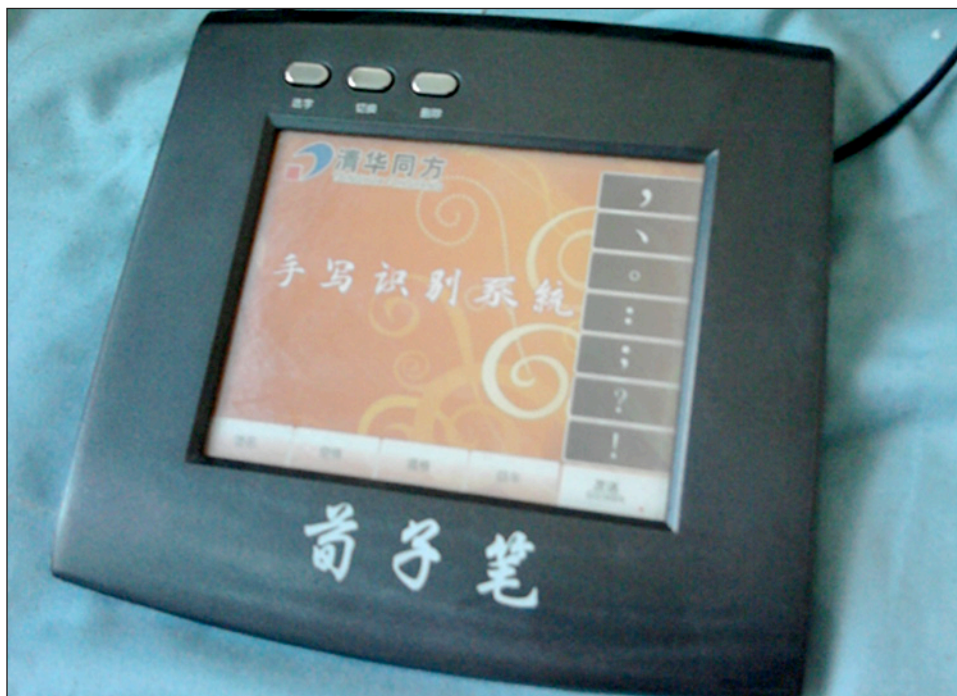
FIGURE 2: A tablet for entering characters using a pen instead of a keyboard.
