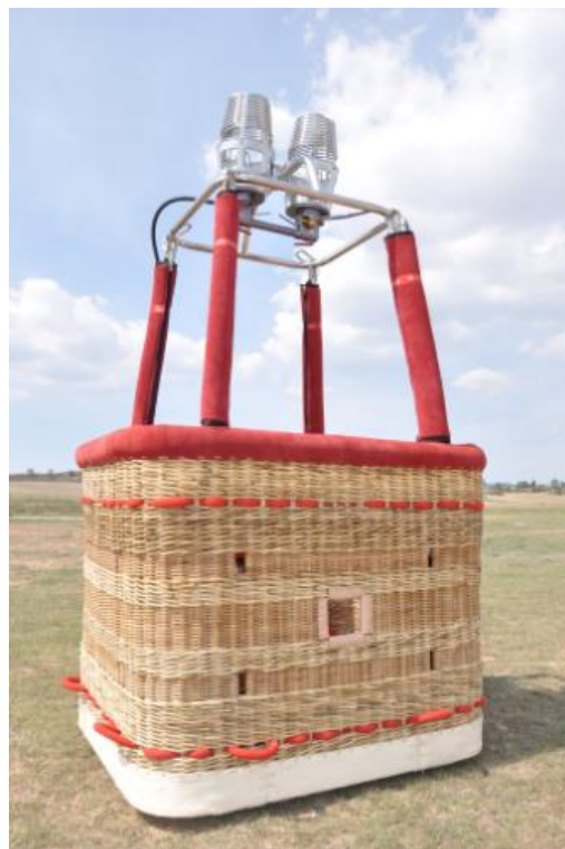
Figure 2. Hot air balloon basket, model C-1 (standard for 2,200 m 3 size balloon)
