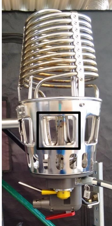
Figure 3. Ultramagic MK-32 single burner
