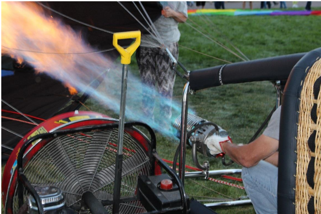
Figure 4. Burner in operation during inflation
