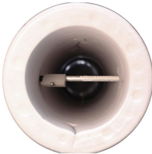
Figure 4.9: Cross section of the duct measurement section, (a) Schematic of the measurement plane, indicating 19 points of measurement; (b) actual setup at measurement location n = 1 ; (c) setup for microphone correlation measurements with microphones at positions n = 4 and n = 16 .
