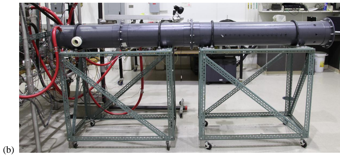
Figure 4.4: Bias flow insertion loss facility (a) schematic; (b) setup.
