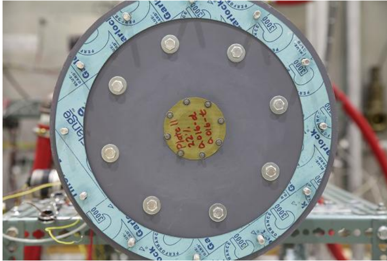
Figure 4.5: Sample mounting plate with perforated plate (Plate 11) attached.
