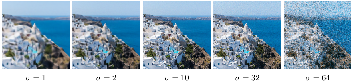
Figure 3.10: A visualization of the 2D image regression task with different Gaussian scales (corresponding to points along the curve shown in Figure 3.9). Low values of \sigma underfit, resulting in oversmoothed interpolation, and large values of \sigma overfit, resulting in noisy interpolation. We find that \sigma = 10 performs best for our Natural image dataset.
