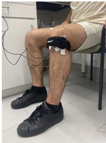
Figure 2. Experimental setup for the knee sound emission portion.
