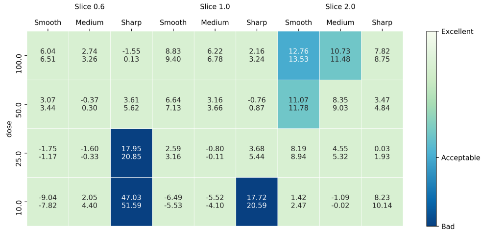
FIGURE 4-13 ACCEPTABLE PARAMETER CONFIGURATIONS FOR PERC15, SCORED ON WFBP WITH BILATERAL FILTERING RECONSTRUCTIONS. NEARLY ALL 95% CONFIDENCE INTERVALS FALL WITHIN THE ESTABLISH \pm 10 HU THRESHOLD. AS SEEN WITH RA-950, THERE IS SOME DEVIATION IN THE “SMOOTHEST” CASES LIKELY CAUSED BY THE DENOISING ALGORITHM.
