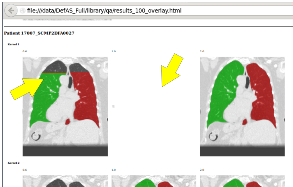
FIGURE 2-17 SAMPLE HTML DOCUMENT, VIEWABLE IN A STANDARD WEB BROWSER. TWO ERRORS ARE CAUGHT (HIGHLIGHTED WITH ARROWS). A FAULTY SEGMENTATION IS SHOWN (TOP OF THE LUNGS IS TRUNCATED IN THE 0.6 MM SLICE) AND A MISSING RECONSTRUCTION OR SEGMENTATION FILE IS CAUGHT VIA THE IMAGE MISSING FROM THE GRID.
