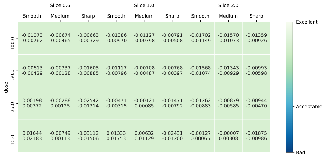
FIGURE 4-5 ACCEPTABLE PARAMETER CONFIGURATIONS FOR WFBP WITH BILATERAL FILTERING APPLIED. ALL 95% CONFIDENCE INTERVALS FALL WITHIN THE ESTABLISH \pm 5\% THRESHOLD.
