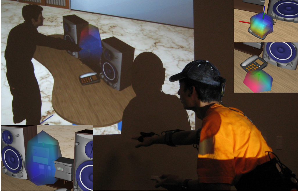
Figure 4.7: Local Coverage Visualization mode. The rendered surface follows the movement of the user's hand, ideal for checking small ROIs.
