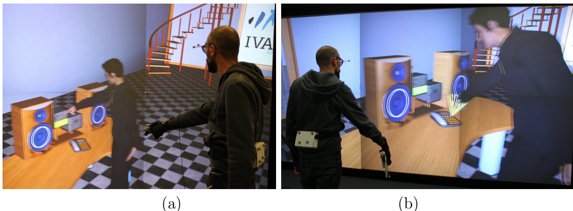
Figure 4.1: (a) In this scenario, during the modeling phase, the user demonstrates several examples of pointing motions in order to demonstrate operations with a stereo system and a telephone. (b) During the training phase, the user requests the virtual human to precisely perform the same pointing motions for arbitrary targets, here specified by the apex of the yellow cone which is controlled via a Wii-Mote controller. The training phase is used here to test if the example motions are sufficiently covering the volume of interest in the scenario. The user can interactively switch between the two phases until all required motions are correctly defined. Note that the simulated images in this figure appear fuzzy since they are being projected for stereo visualization.
