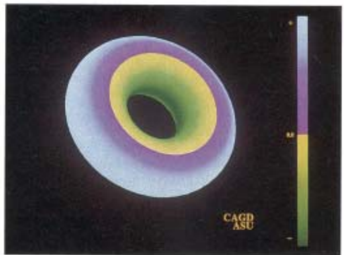
Figure 9. Gaussian curvature used as a texture.
