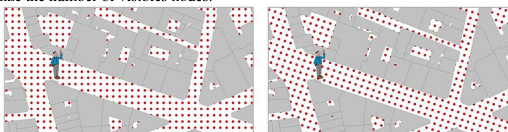
Figure 5: Initial grid before (left) and after optimization according to the street orientation where observer is located (right)
