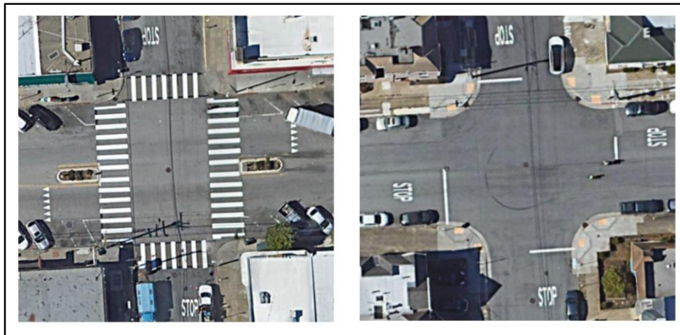
Figure 1: Satellite imagery of intersections in San Francisco with (left) and without marked crosswalks (right).
