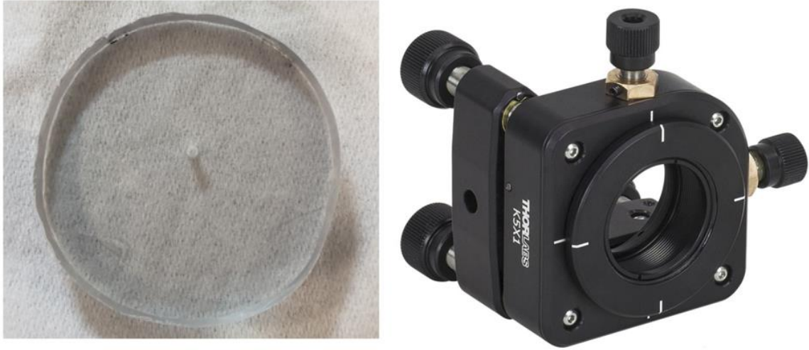
Figure 9. On the left is the 3mm polycarbonate phase plate that was made in our lab. The pinhole in the center was drilled with a 0.9mm drill bit. The resulting phase plate was put into a 5 axis kinematic base that is shown on the right.
