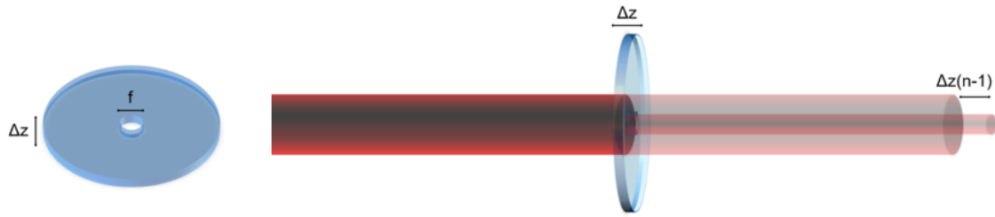
Figure 6. Visual representation of a phase plate. It should be noted that the phase delay is introduced by the difference in the index of refraction between the phase plate material and air.
