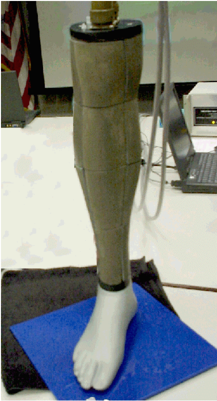
Figure 16: Sixteen Segment Thermal Manikin Calf
