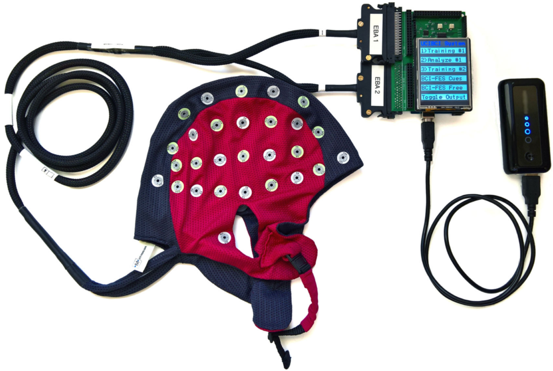
Fig. 1. A picture of our BCI system with an EEG cap and a portable 5V battery. The BCI system and battery cost <$200. The touchscreen, with built-in microSD slot, acts as the user-interface for the BCI system and eliminates the need for a monitor and keyboard. It snaps onto a shield with the custom amplifier array which snaps onto a commercial microcontroller. EEG signals are amplified by the custom array and sent directly to the microcontroller for processing, BCI decoding, and effector output.
