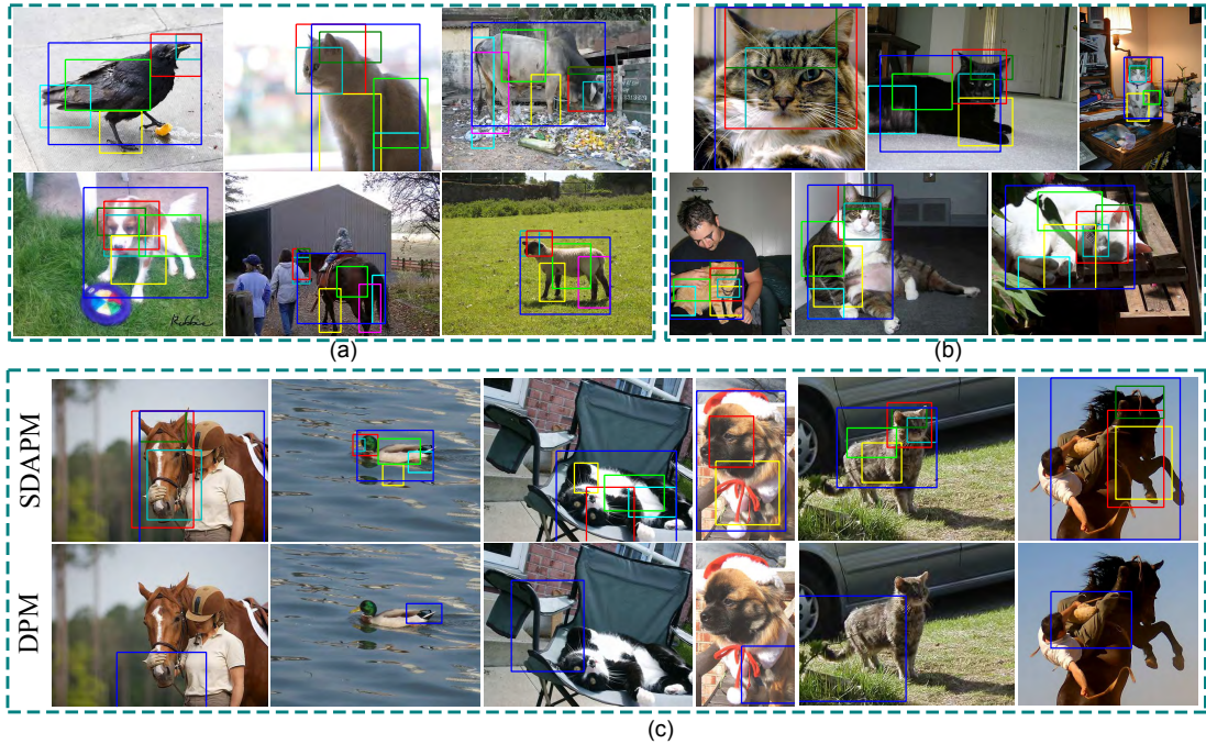
Figure 5.2: Our method provides a richer object representation and improves the detection results. The blue bounding boxes correspond to the whole object detection, and boxes of other colors correspond to semantic parts respectively, which may indicate different parts across classes. (a) shows one representative result for each of the six animal classes. (b) shows detection results of the cat class to illustrate the ability of our model to robustly represent objects under non-rigid deformations, viewpoint changes, and occlusions. (c) shows typical examples that are correctly localized by our Scene-Domain Active Part Model (SDAPM) but missed by DPM.
