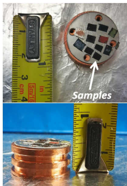
Figure 1: The sample holder and pasted samples. The sample holder is a copper cylinder with a height of 0.5 inches and a diameter of 1.0 inches. The samples are typically several mm in size. Please click here to view a larger version of this figure.
