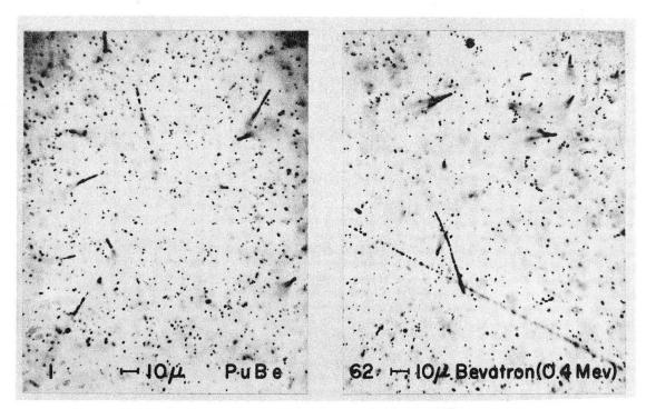
NTA films | and 62 Exposure |: |.4 x 10<sup>8</sup> <u>neutrons</u> 62: 3.2 x 10<sup>8</sup> <u>neutrons</u> cm<sup>2</sup> Dose~6 rem in each case
