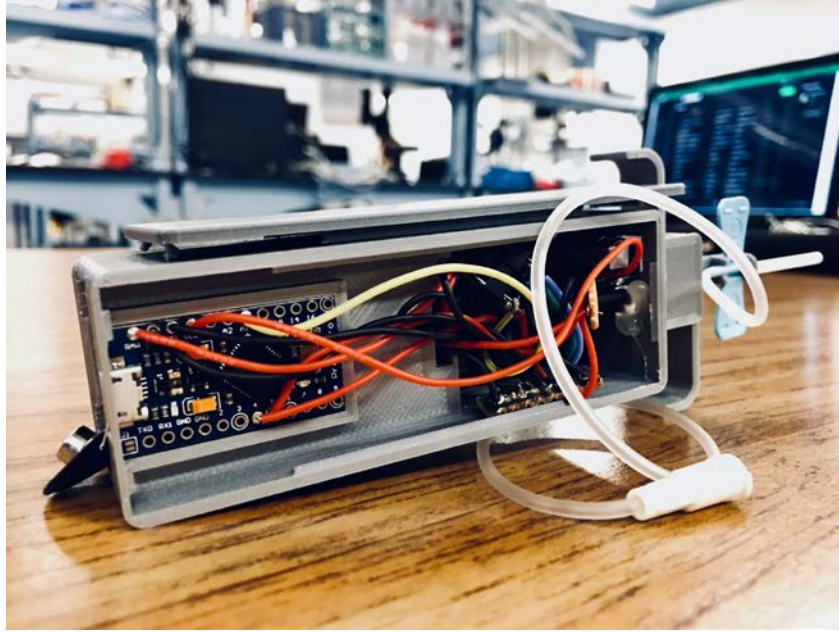
Figure 4: Full design of our prototype with force sensing apparatus, vacutainer holder, and casing.
