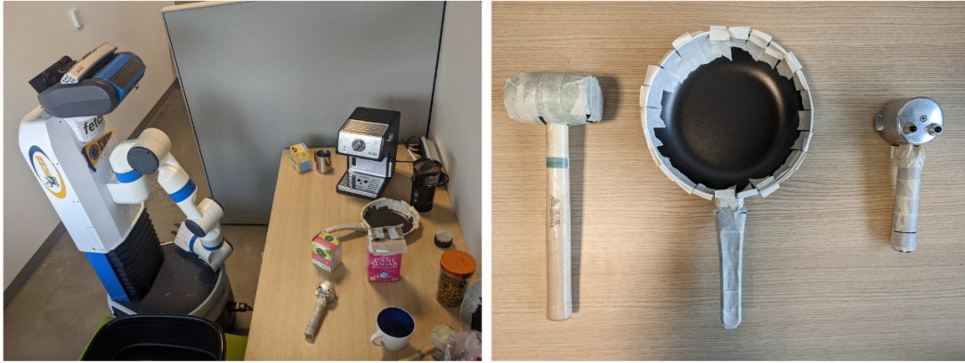
Figure 4.1. Left: the setup of the real-world experiment with Fetch. Right: Objects (hammer, pan, and espresso machine handle) used in the real-world experiment.
