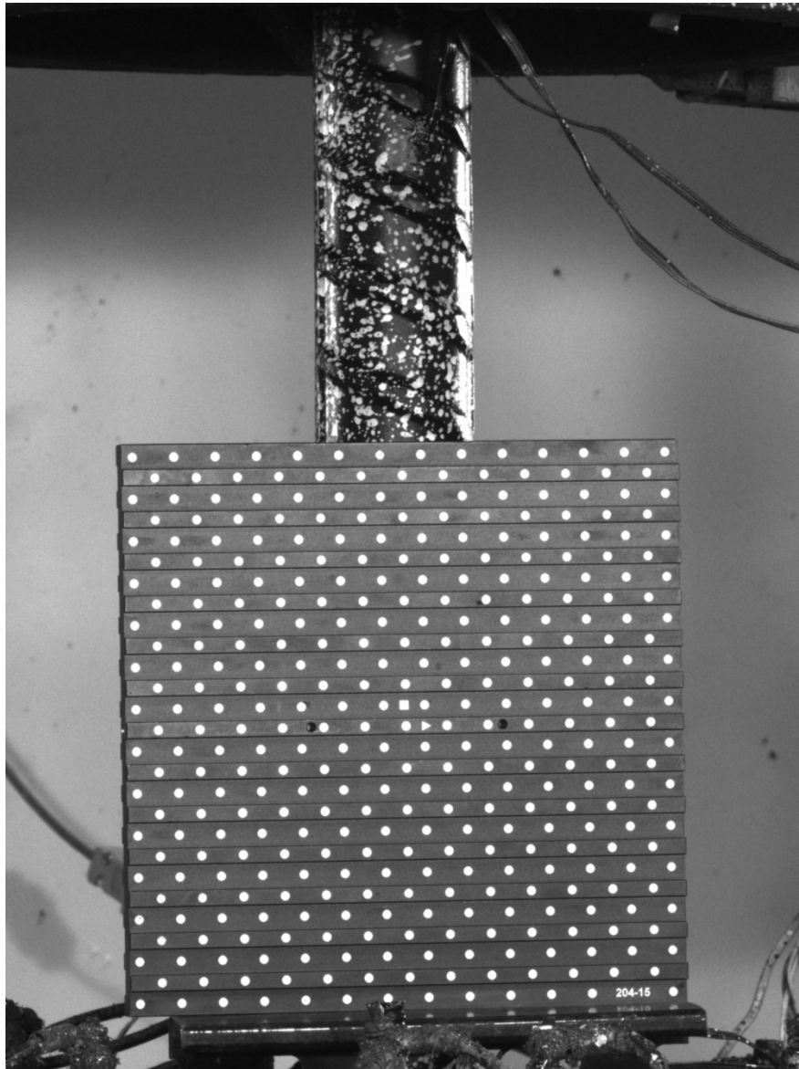
Figure 3.16. Calibration plate for DIC post-processing.
