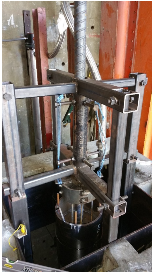
Figure 3.20. Upper pipe grip (no SC) inside heat transfer fluid tank with test bar and removable aligning frame.
