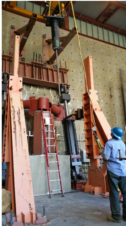
Figure 3.22. Transfer of upper pipe grip from heat transfer tank into loading apparatus.
