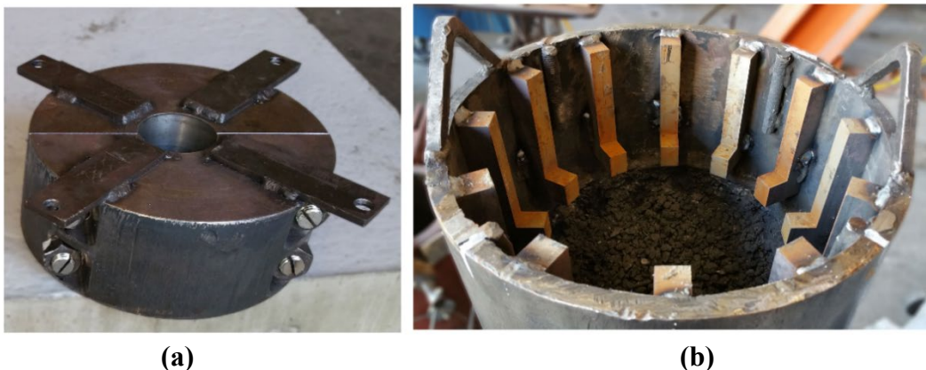
Figure 3.10. (a) Circular steel plate; (b) L-shaped support brackets for steel blocks.
