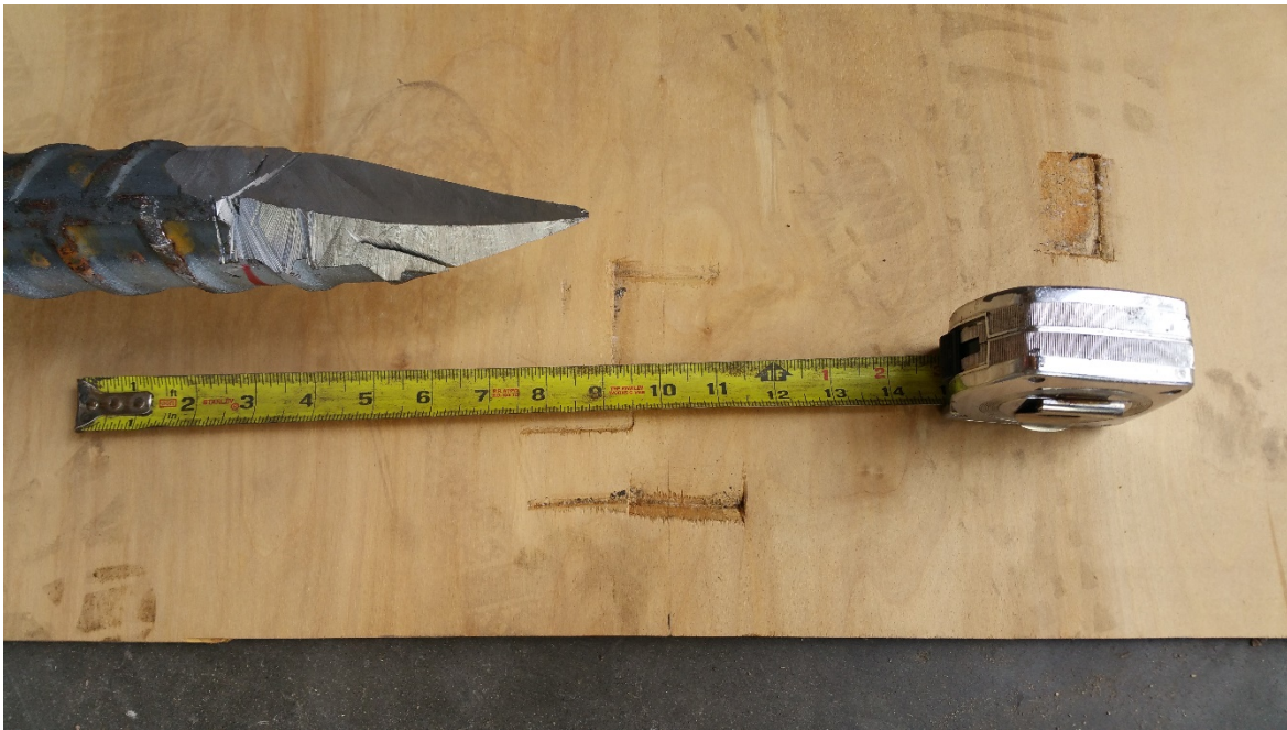
Figure 3.26. Bar end cut into spear head.
