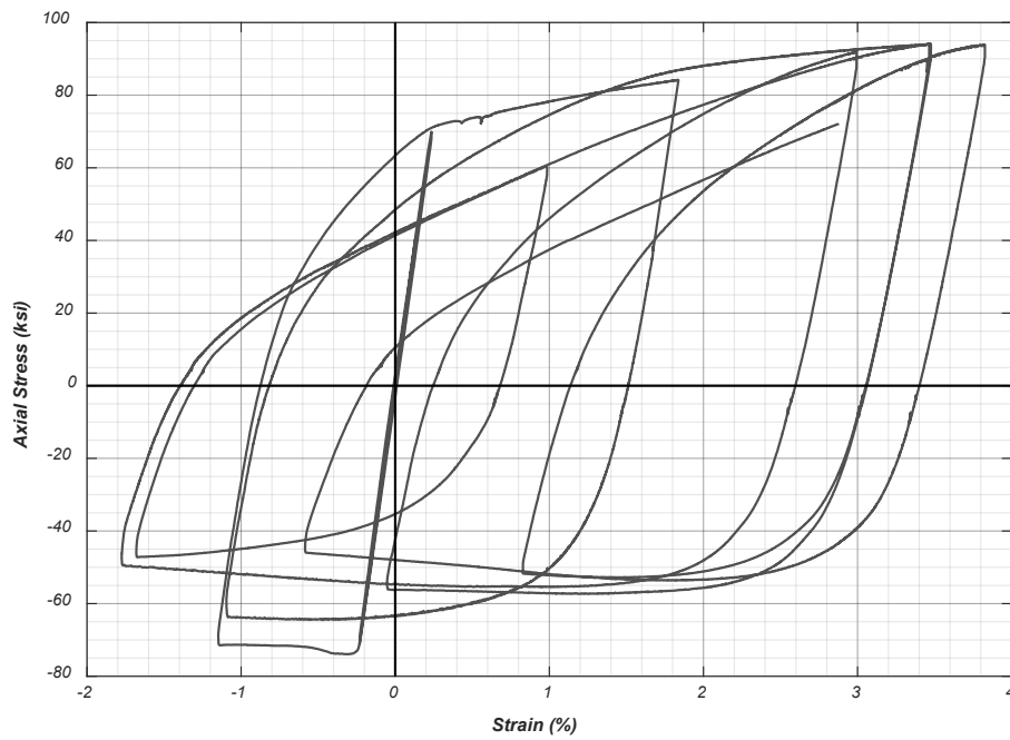
Figure 3.46. Axial stress-strain response of No. 18 bar with unsupported length of 8d_b subjected to random history cycles (Specimen19).
