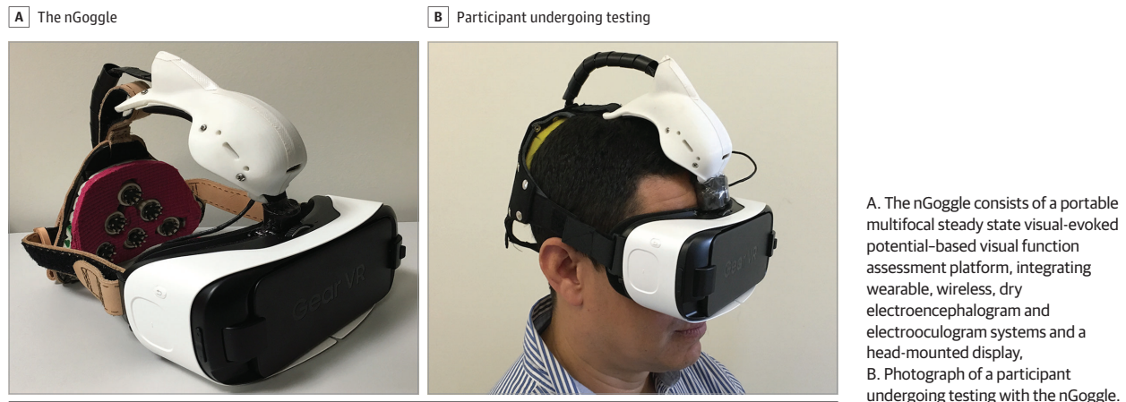
Figure 1. The nGoggle, a Portable Brain-Computer Interface for Assessment of Visual Function
