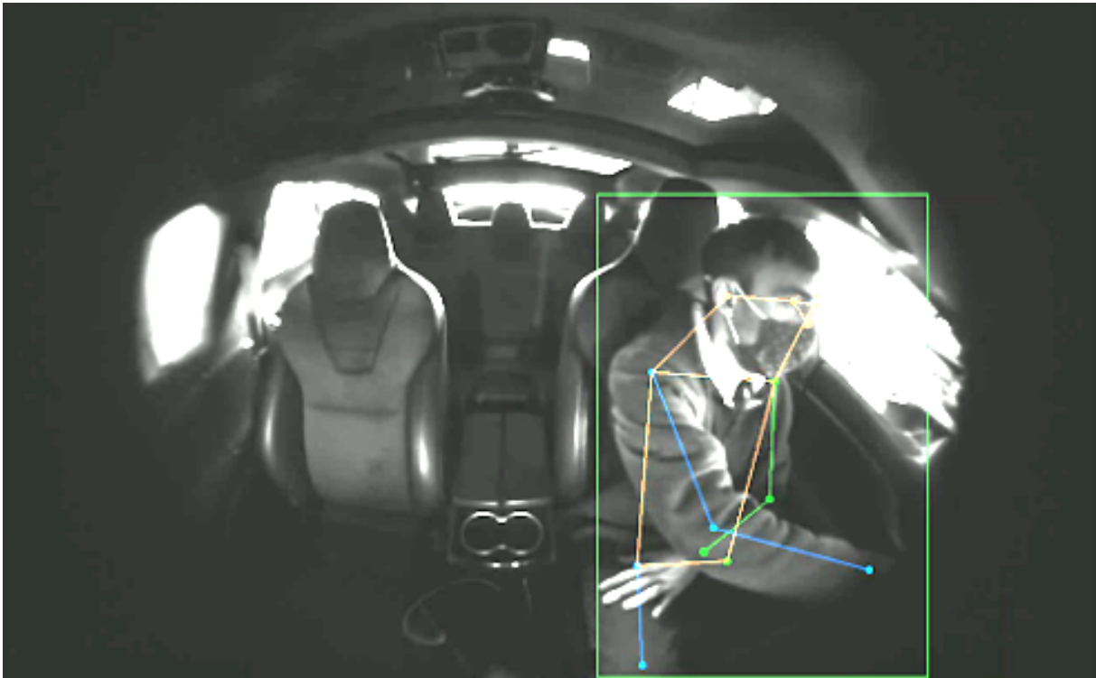
Figure A.7. Prior to classifying driver hand activity, the system must detect the driver. We use Faster-RCNN to generate the bounding box shown in green. Following driver detection, we apply HRNet to identify the 2D pose skeleton, shown as keypoints and connecting lines on the driver's body.
