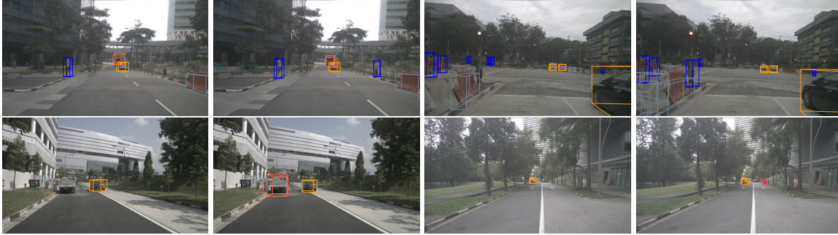
Figure 5.1. Choosing the most informative data can impact object detection model performance. Images in the left column are the results of a model trained on 50% of nuScenes data, selected at random. Images in the right column are the results on the same images of a model trained on 50% of nuScenes data, but selected using our VisLED active learning query strategy. In the top two rows, we see cases where challenging pedestrians are missed on the left image (preparing to cross on the right side of the road, and standing behind the crossing pole, respectively), but correctly detected on the right. Similarly, in the bottom two rows, the under-represented classes of motorcycle and truck are more readily detected using our active learning strategy.
