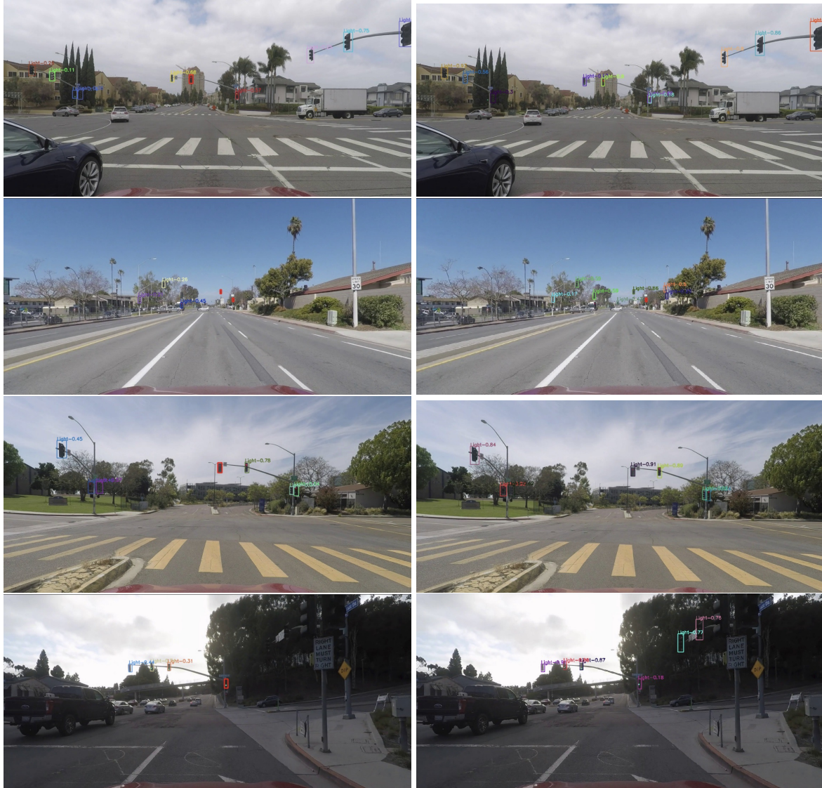
Figure 11.7. Qualitative results of training without salience-sensitive loss (left) and with salience-sensitive loss (right). In each example, a red border is given to signs which are “missed” by the detector. In these examples, the missed sign is salient and critical to the car’s decisions. These signs are sometimes further or smaller than other signs in the scene, making salience an important part of the training process since the “easiest” signs may not be the most important to the vehicle’s planning.
