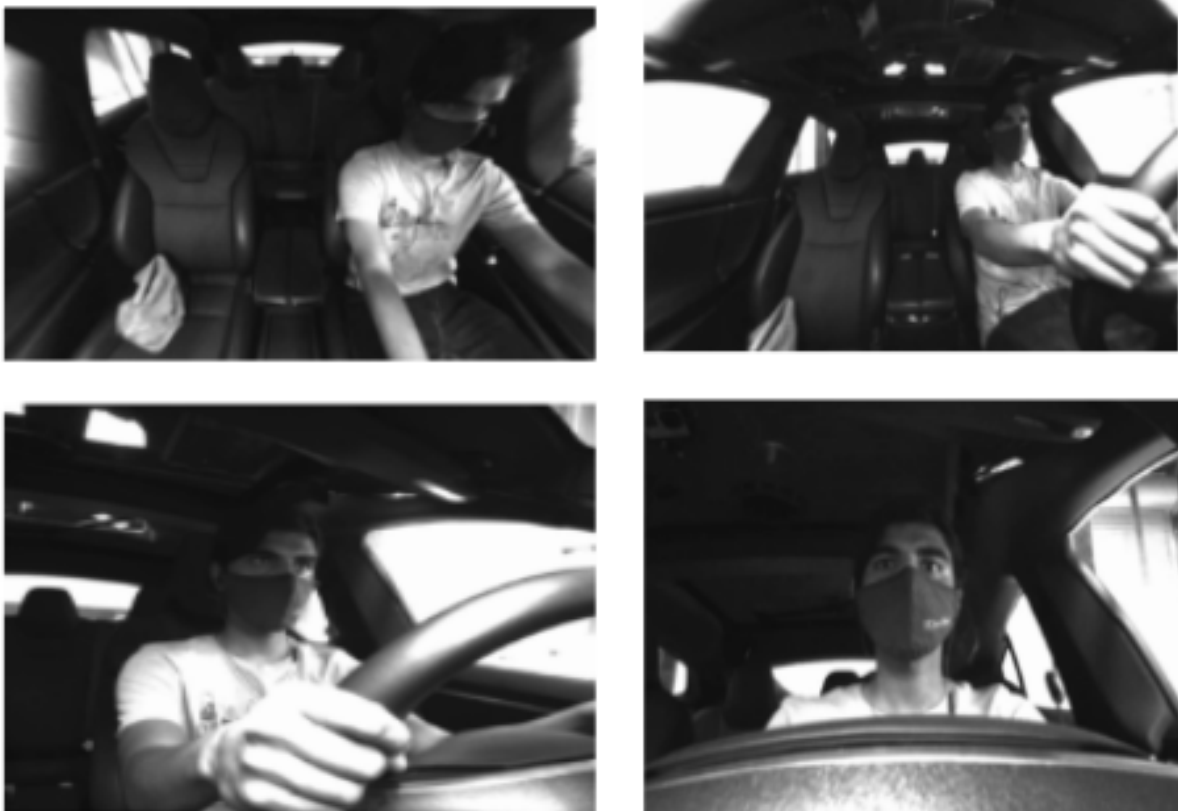
Figure A.1. Multi-view images (clockwise) - rearview, dashboard center, steering view, and dashboard driver, which explain how hands can be missing in certain frames, causing an irregular redundancy .
