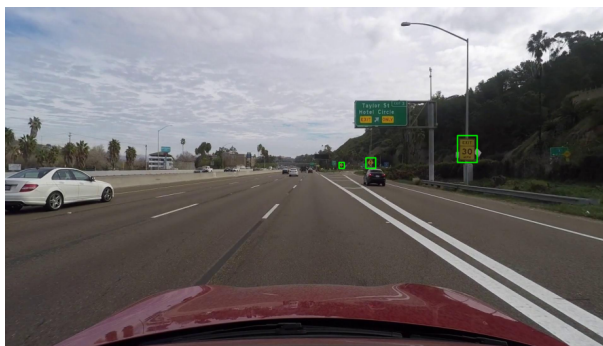
Figure 9.4. While most speed limit signs apply to all lanes in the direction of travel, this exit speed limit applies only to the lane to the right of the ego vehicle. An autonomous vehicle must have the ability to determine whether this sign is salient to its lane, and select its speed accordingly. The detected signs in this scene are not salient.
